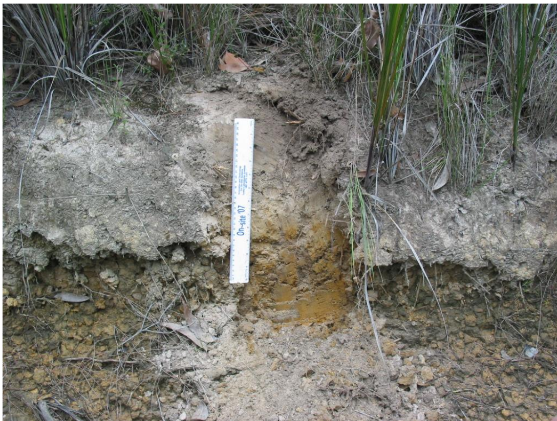
Figure 8 - Photo showing exposed soil profile in table drain along Advance Road. Note evidence of dispersion and erosion of B horizon (clay subsoil)
