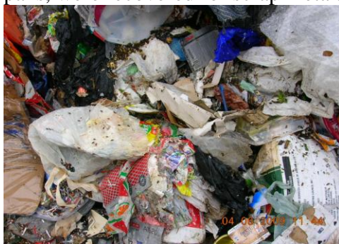
This shows bag damage caused by compaction and broken glass.
