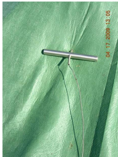
1200mm Compost temperature probe insert through Compostex Cover
