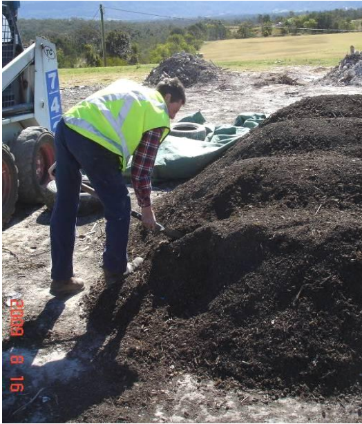
1. Samples were removed from throughout the pile.
