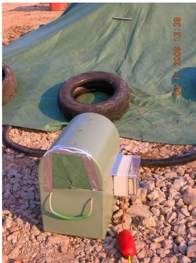
Forced Aeration Fan Control Unit, with 750 W fan and thermostat controlled switch
