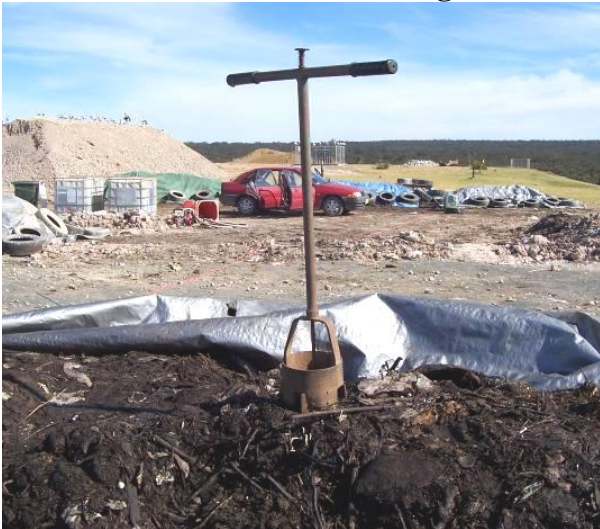
Post hole digger used to take the core samples. Pictured right-a close up of 450mm sample.
