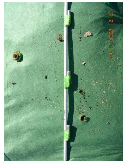
Temp Data Loggers taped to conduit. This was inserted into the compost piles to log temperature through the pile.
