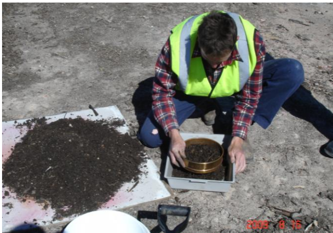
3. The material was sieved with a 16mm screen.
