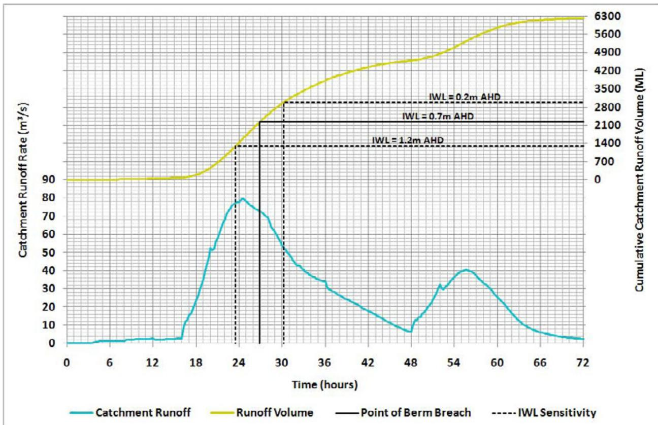
**Figure 6-9 Sensitivity of the April 1988 Event Simulation to Initial Lake Water Level**
