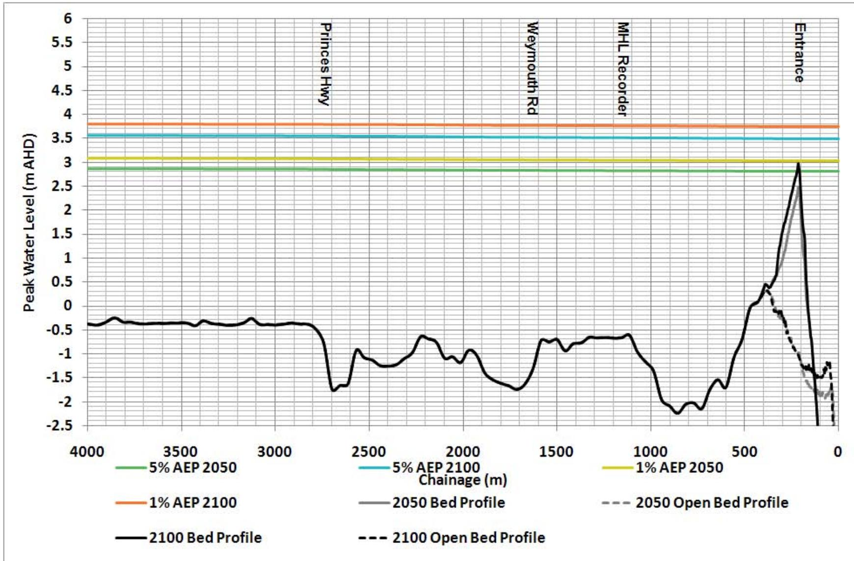
Figure 8-10 Design Flood Level Profiles for Ocean Derived Events Incorporating Future Climate Change Predictions
