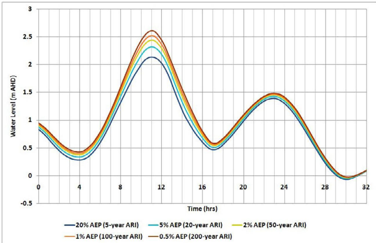
Figure 7-4 Design Ocean Boundaries for Ocean Flood Events
