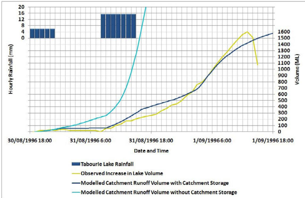
**Figure 6-5 Comparison of Simulation and Observed Lake Response September 1996**
