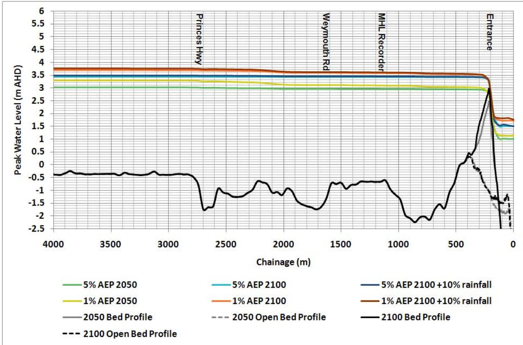
Figure 8-9 Design Flood Level profiles for Catchment Derived Events Incorporating Future Climate Change Predictions
