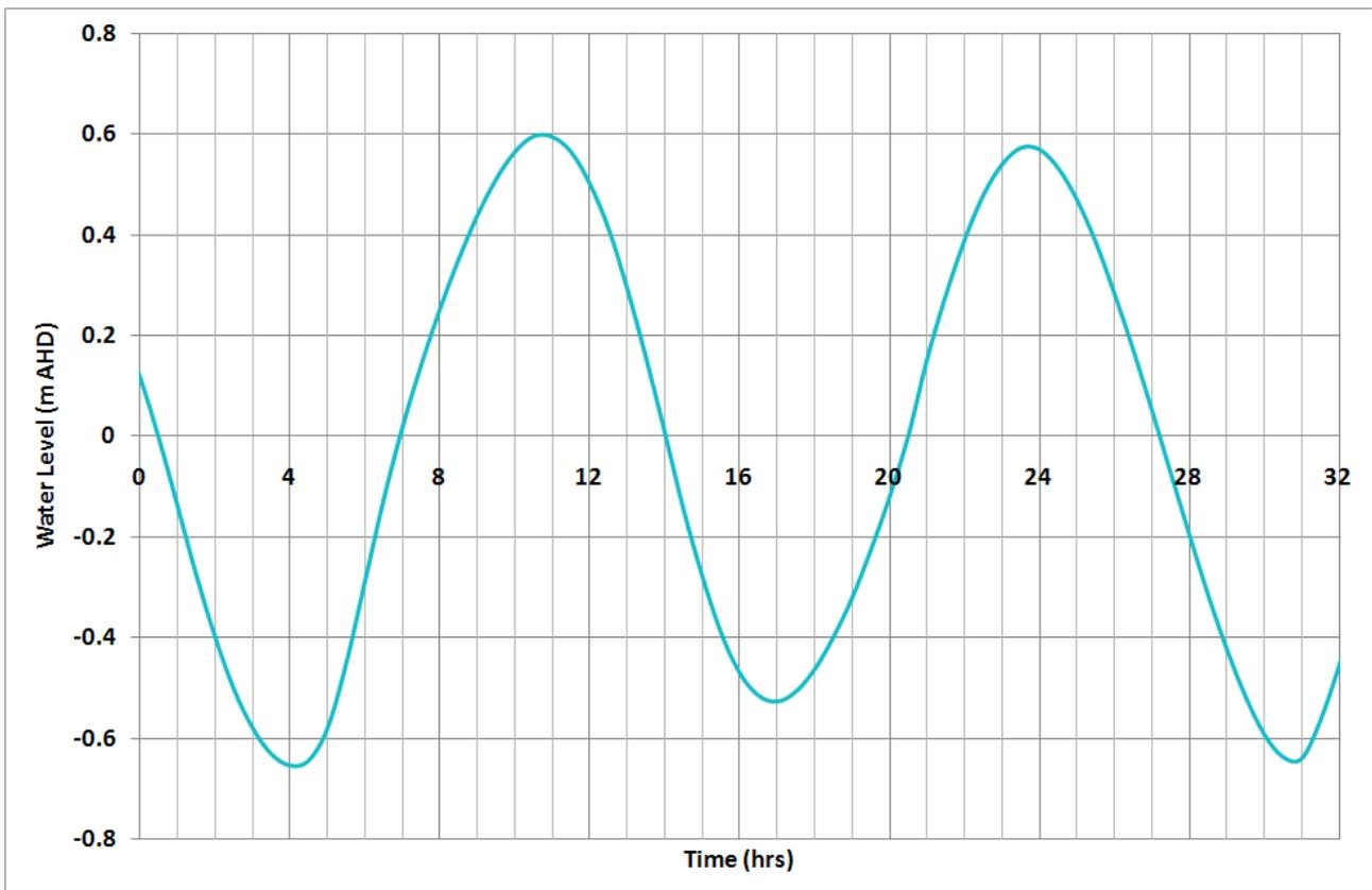
**Figure 7-2 Design Ocean Boundary – Regular Neap Tide**
