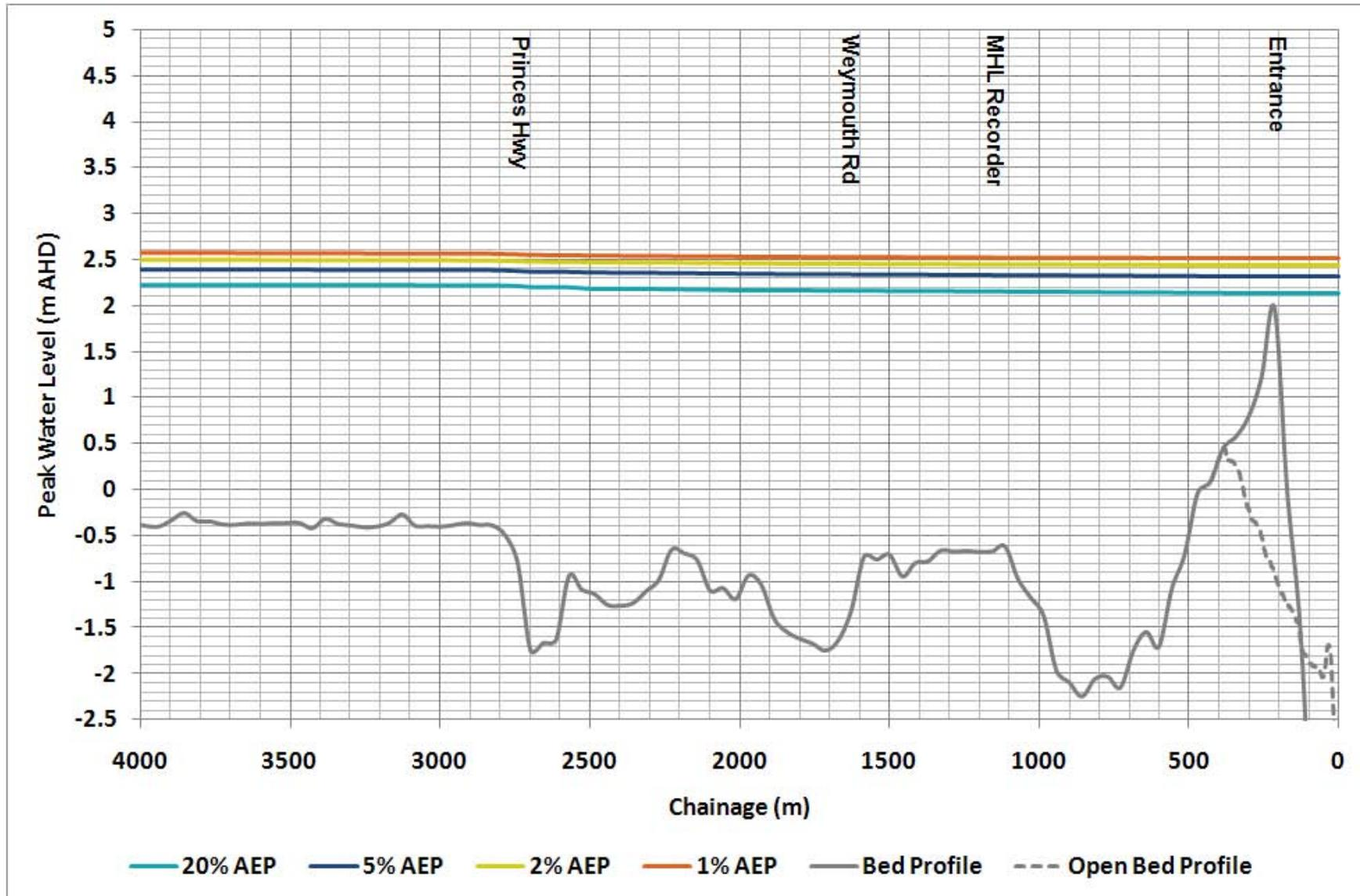
Figure 8-4 Design Flood Level Profiles for Ocean Derived Events
