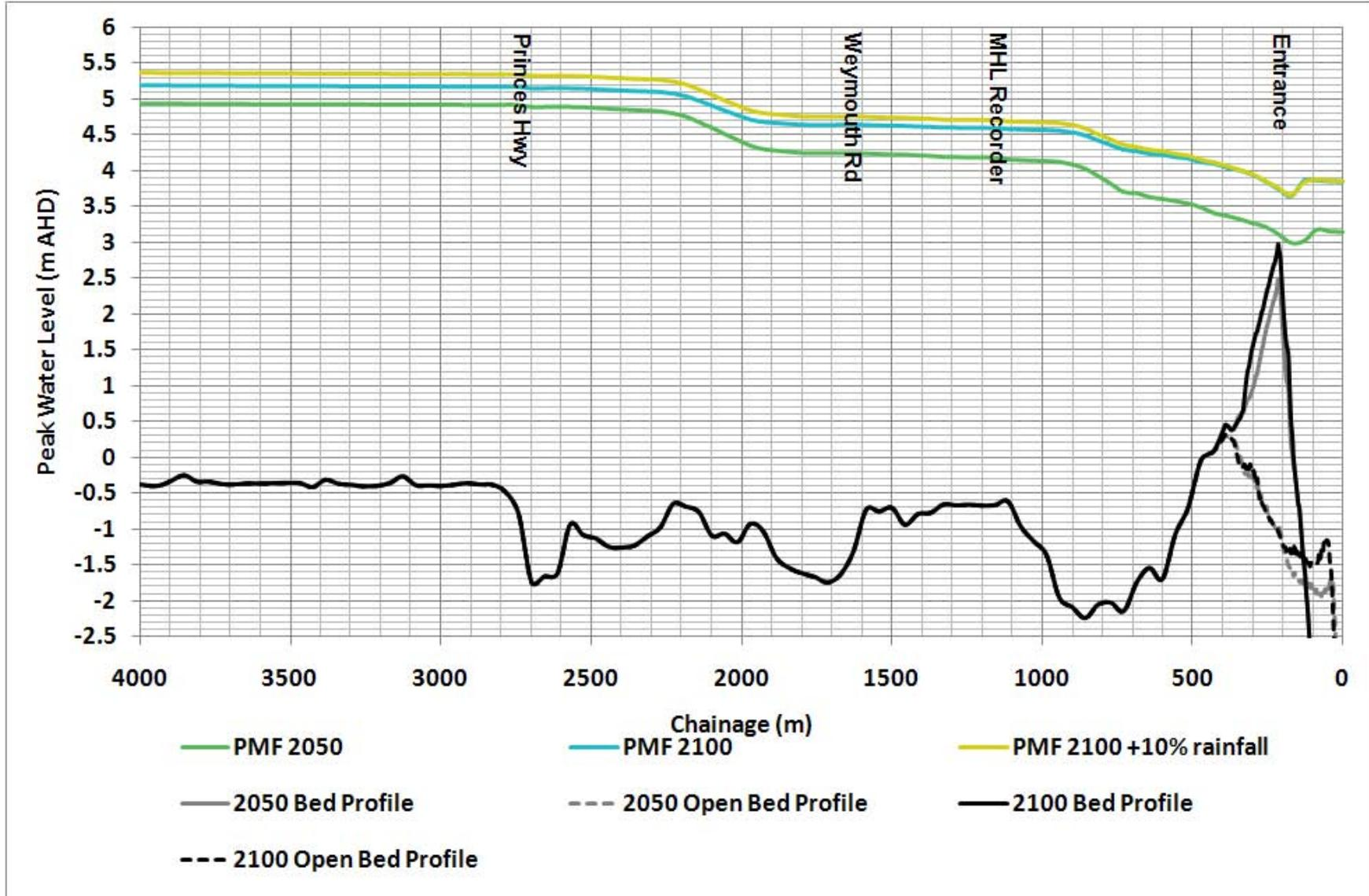
Figure 8-11 Design Flood Level Profiles for PMF Events Incorporating Future Climate Change Predictions
