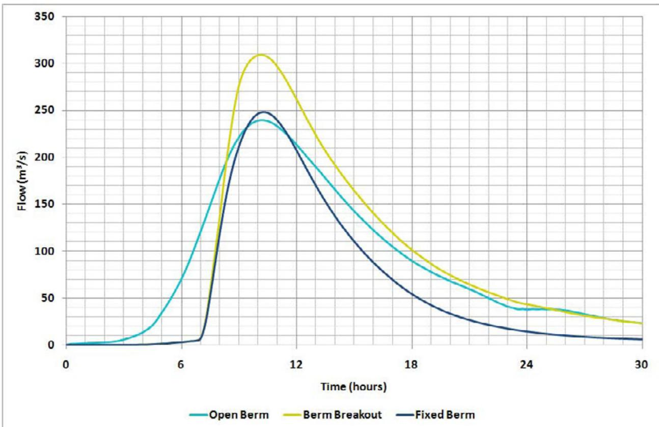
Figure 8-8 Impact of Entrance Condition on Catchment Derived 1% AEP Flow Hydrograph
