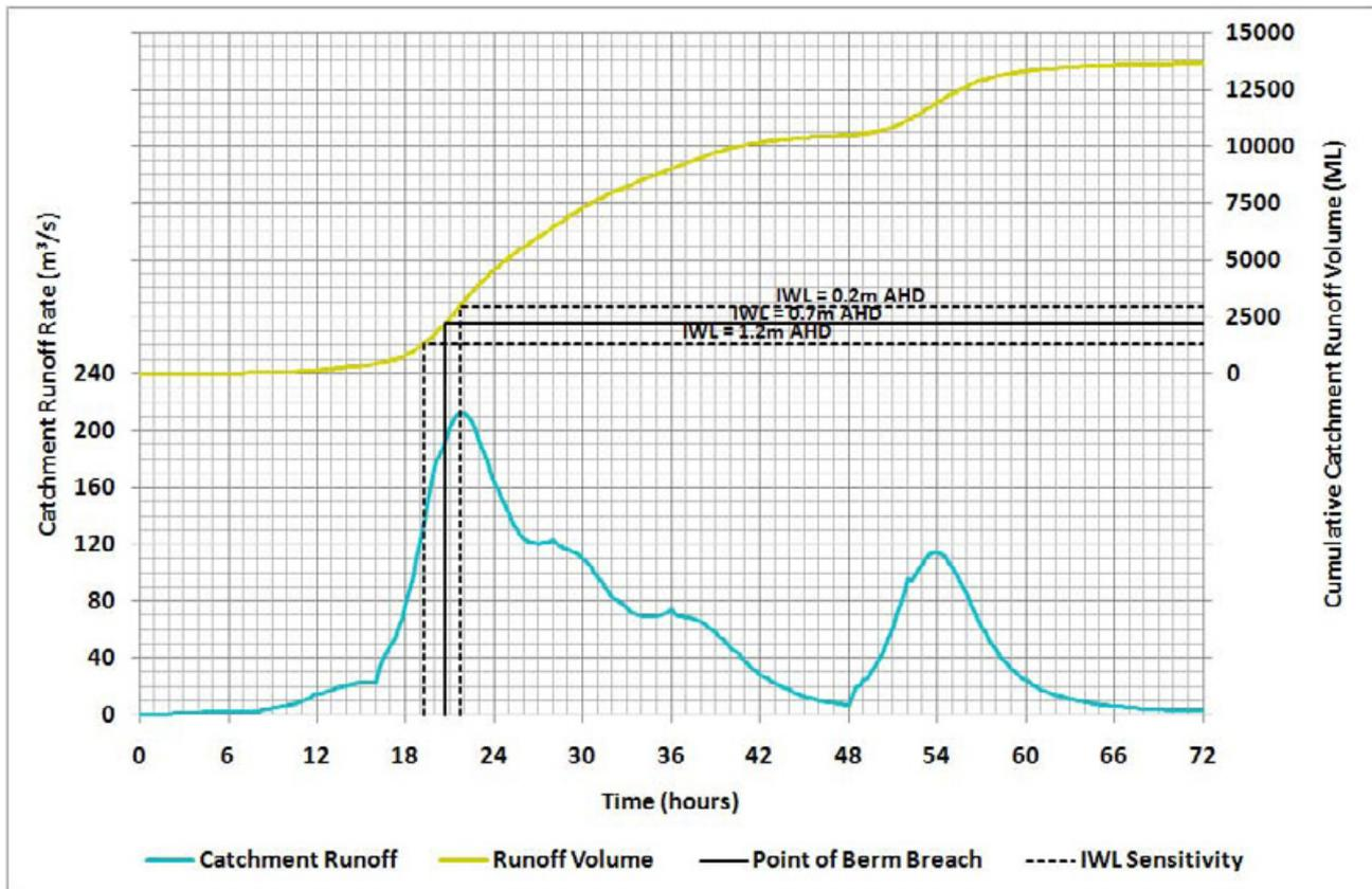
**Figure 6-8 Sensitivity of the March 1975 Event Simulation to Initial Lake Water Level**
