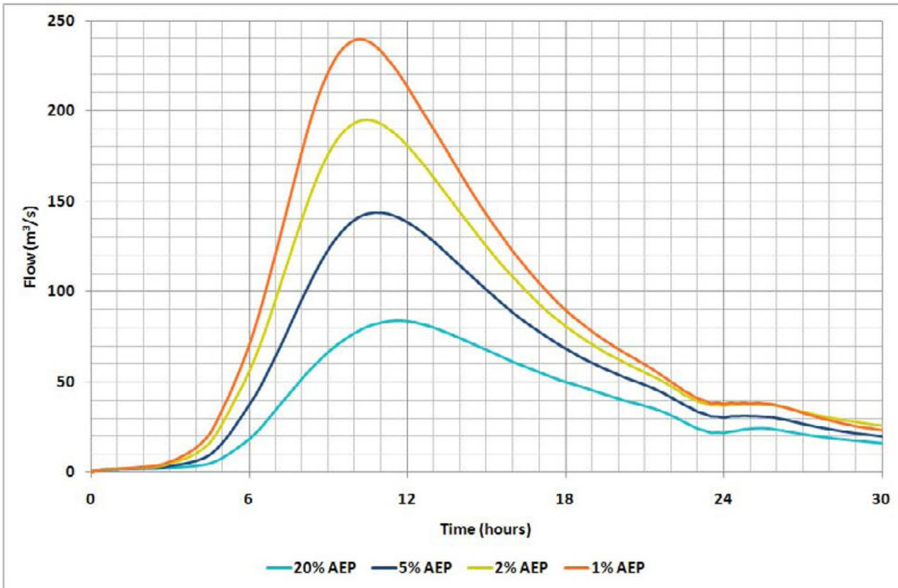
Figure 8-6 Catchment Derived Design Flood Hydrographs for Tabourie Lake Entrance
