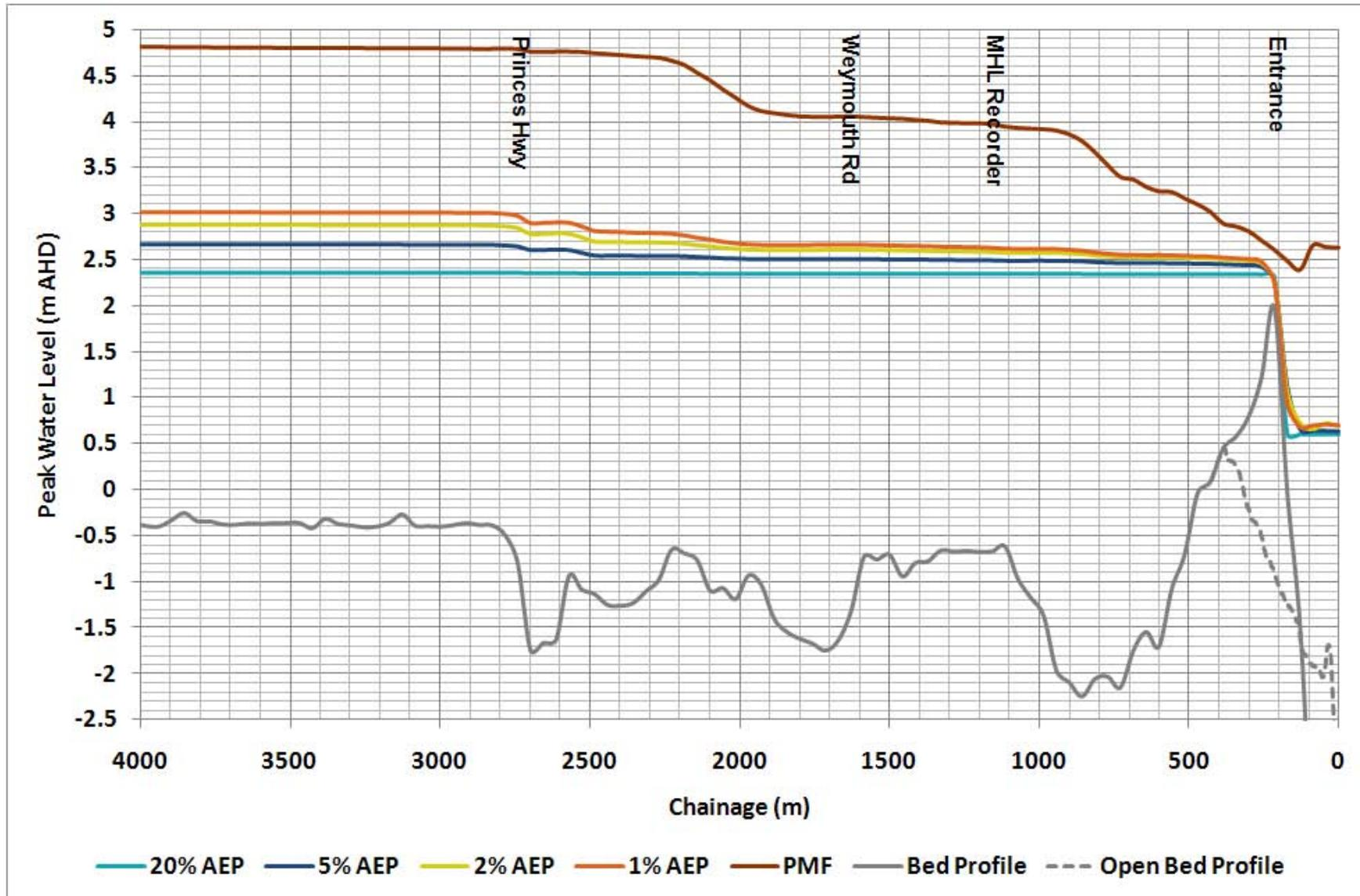
Figure 8-1 Design Flood Level Profiles for Catchment Derived Events
