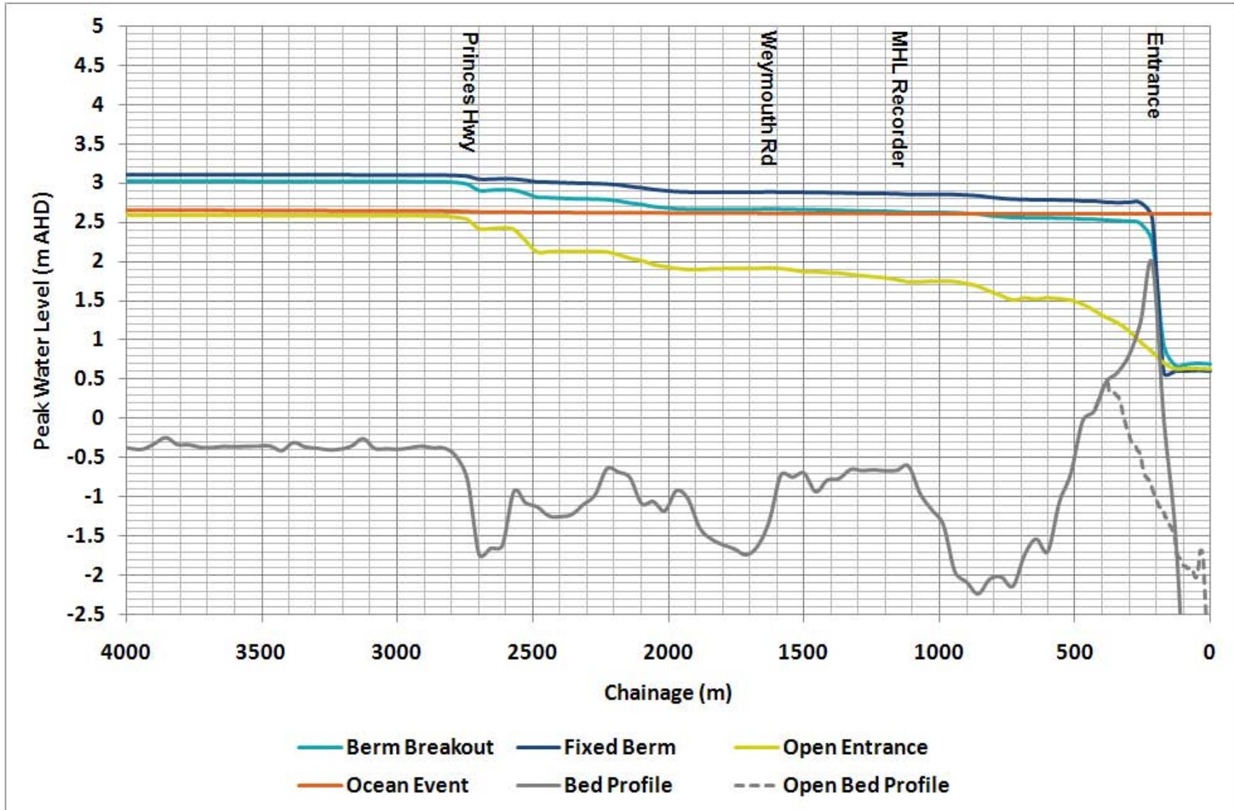
Figure 8-2 Design Peak Flood Level Profiles for the 1% AEP Event
