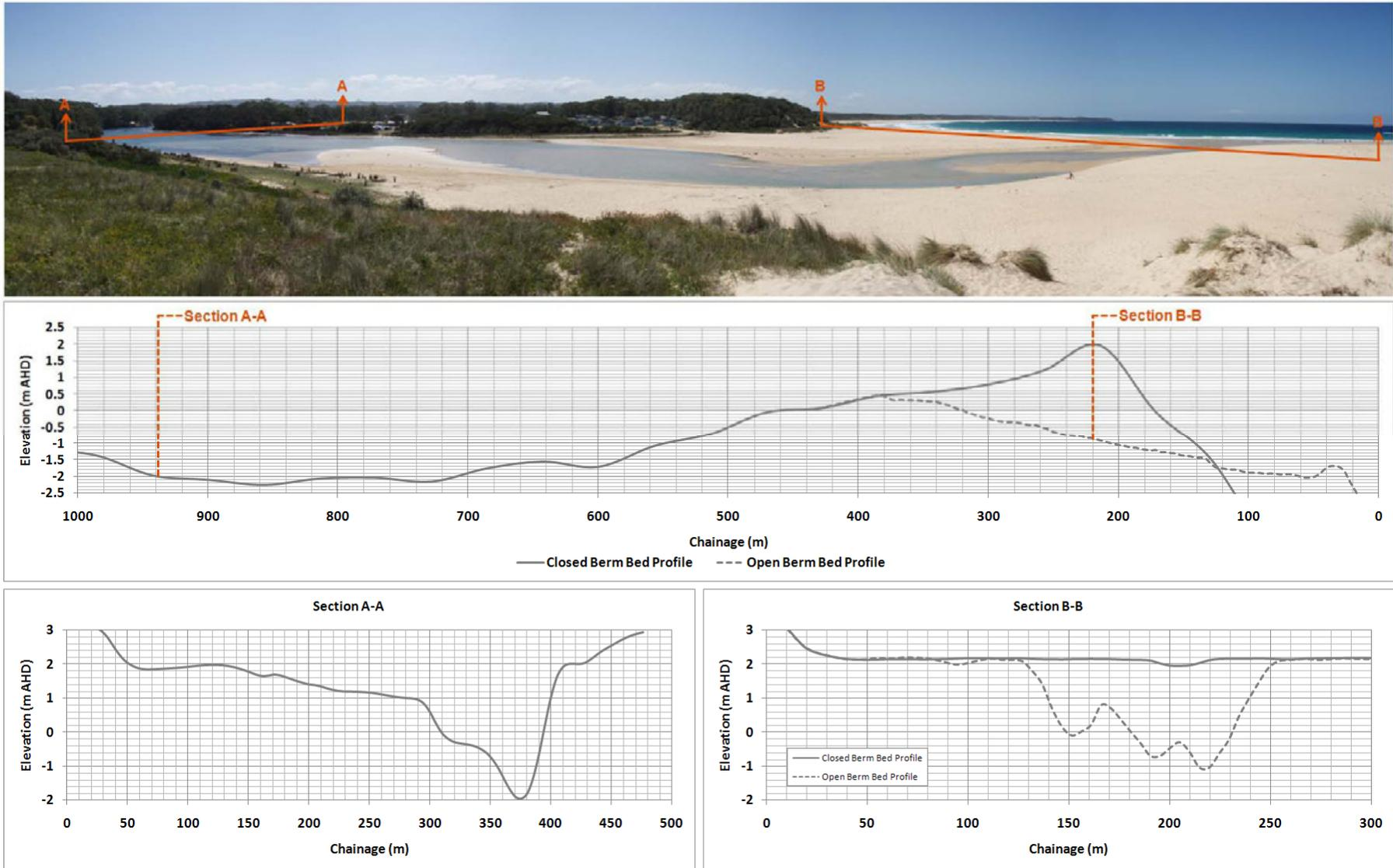
Figure 7-5 Design Berm Geometry
