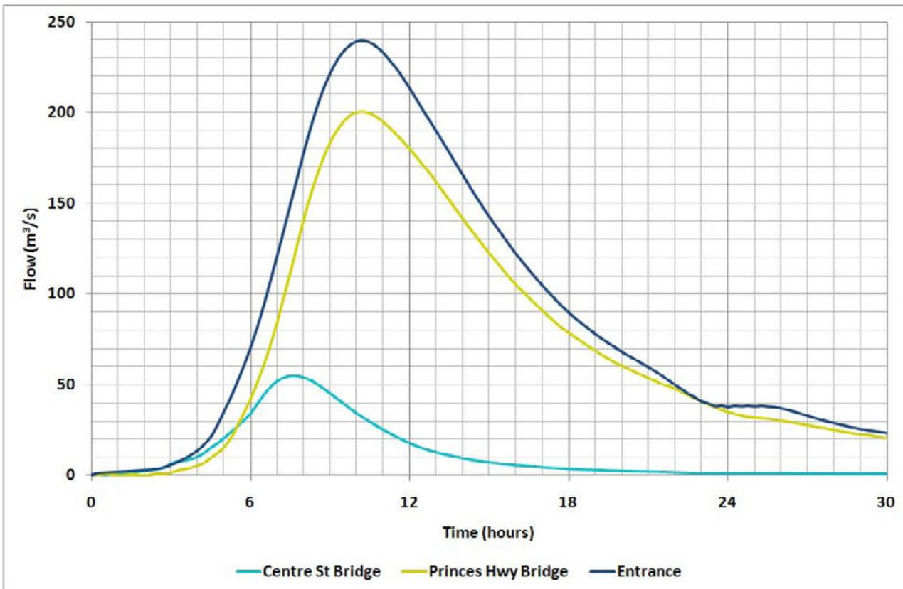
Figure 8-7 Timing of Catchment Derived Design 1% AEP Hydrographs for Tabourie Lake
