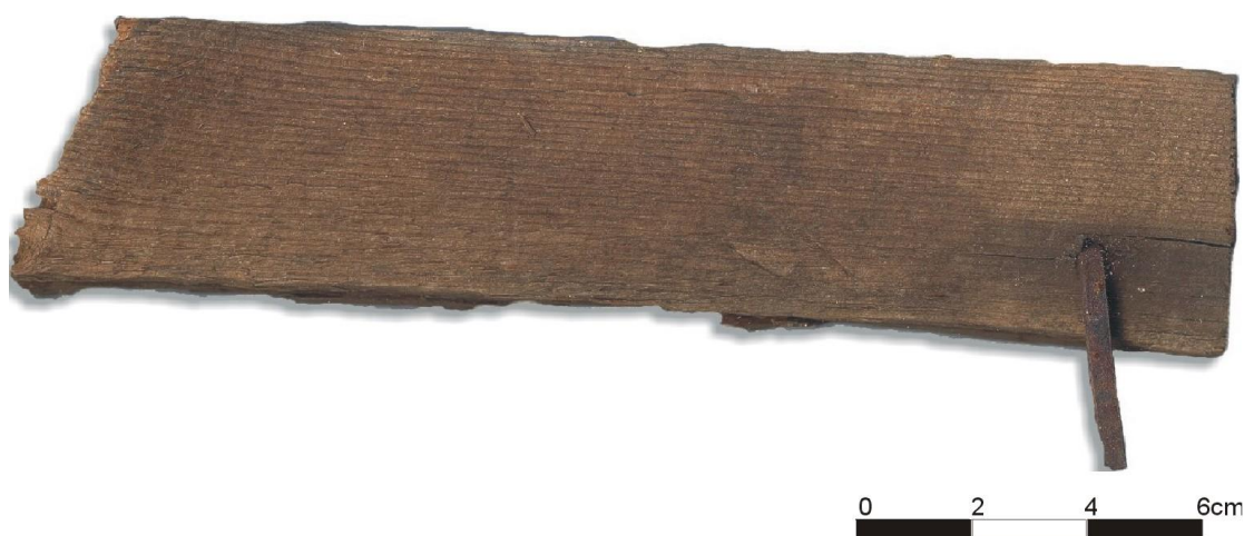
Figure 6: A remnant of a cedar batten with nail from roof of Graham Lodge .
