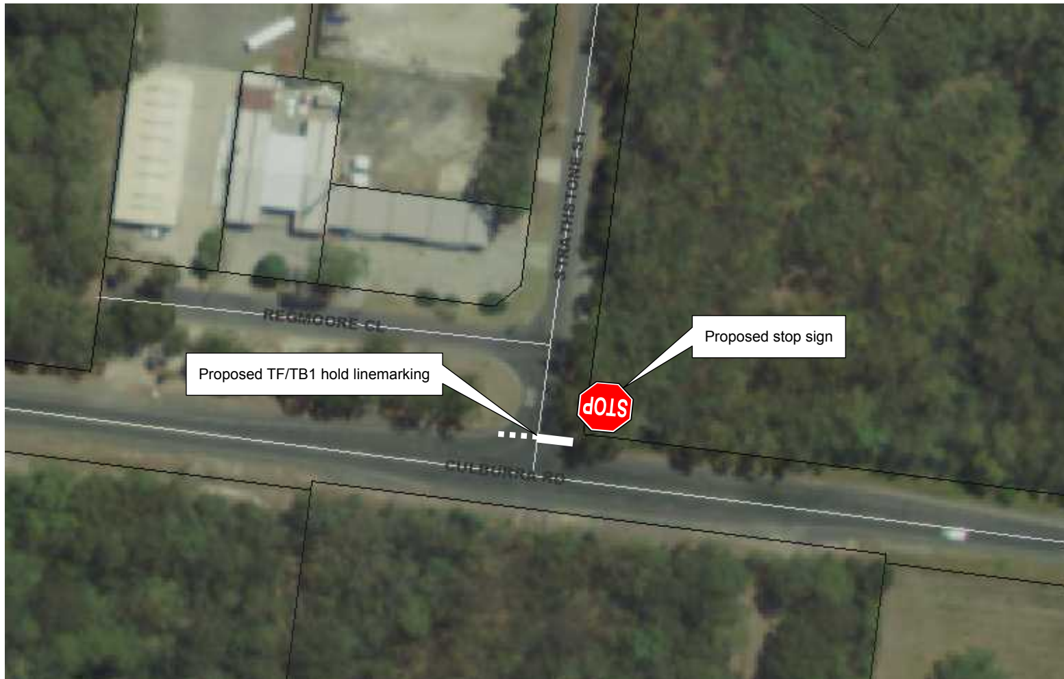
Proposed stop sign and hold linemarking Intersection of Strathstone St and Culburra Road, Culburra
