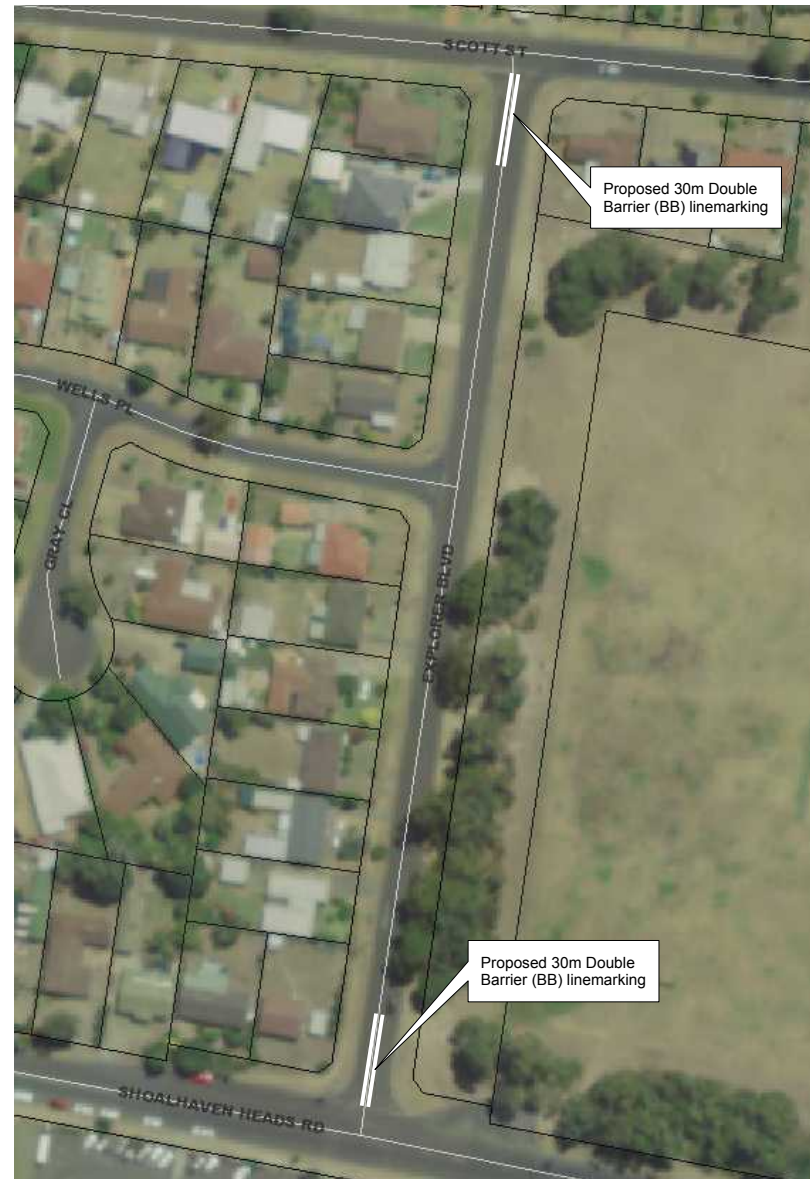
Proposed Double Barrier (BB) linemarking Intersection of Explorer Boulevard and Scott Street Intersection of Explorer Boulevard and Shoalhaven Heads Road, Shoalhaven Heads
