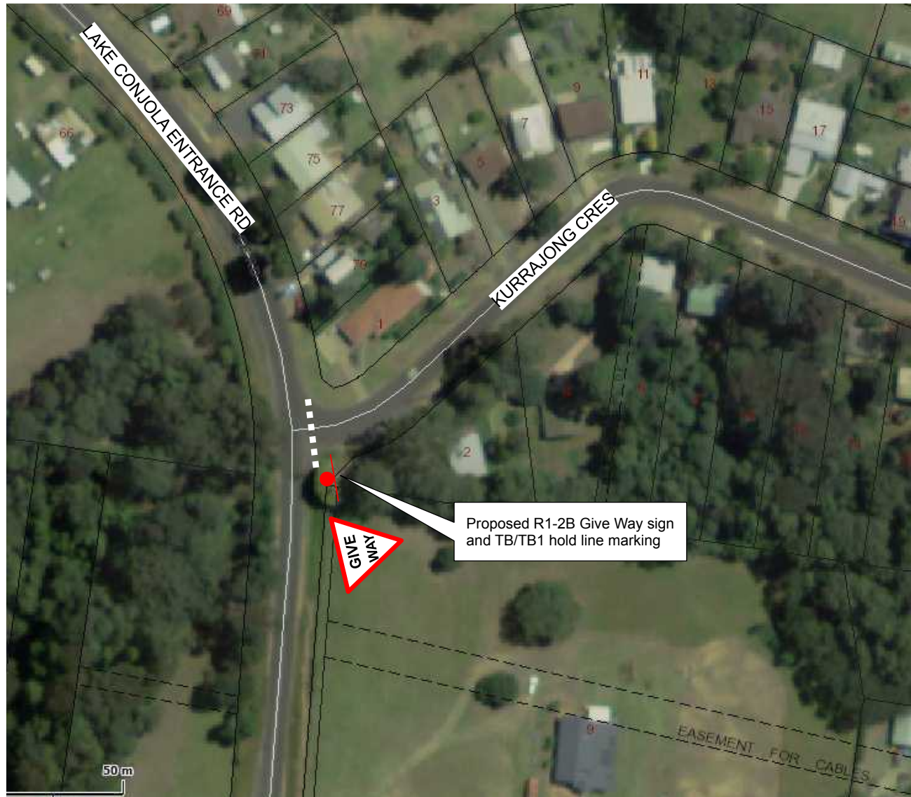
Proposed Give way sign and associated hold linemarking intersection of Kurrajong Cres and Lake Conjola Entrance Rd
