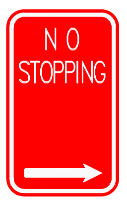
R5-400 (R) SIGNPOSTING DETAIL A NOT TO SCALE
