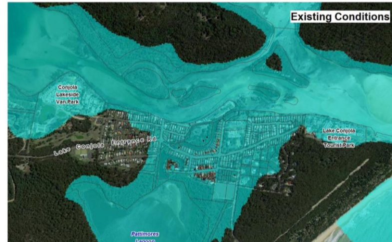
Existing 1 in 100-year flood extent in Conjola Lake showing extensive potential property inundation
