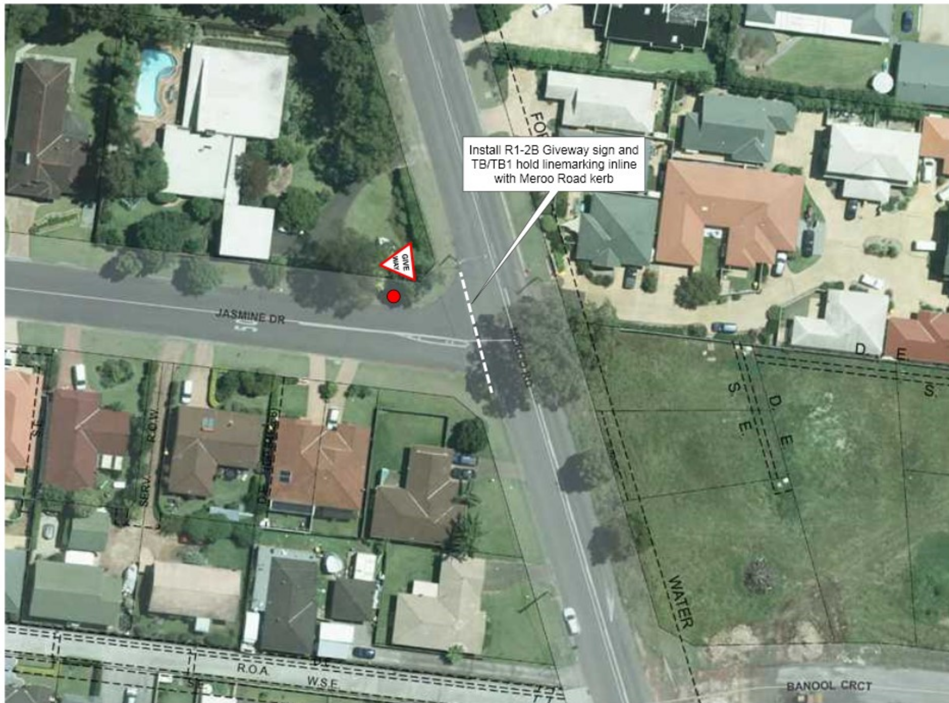
Install Give Way sign and hold line Intersection Jasmine Drive and Meroo Road, Bomaderry
