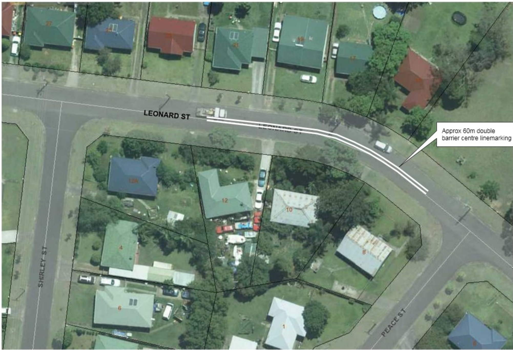
Proposed Centre Linemarking Lenard St, Bomaderry
