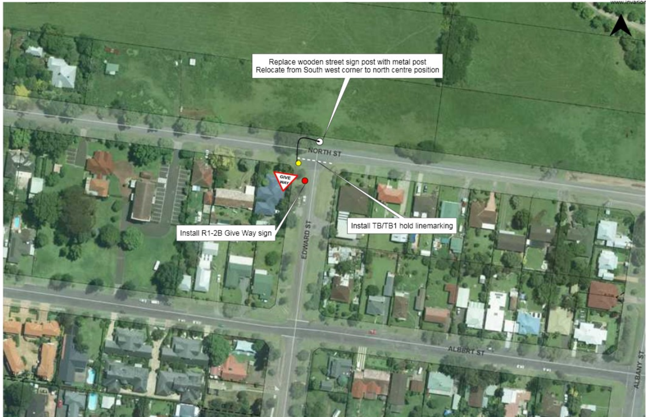
Install Give Way sign and hold line Intersection of Edward Street and North Street, Berry
