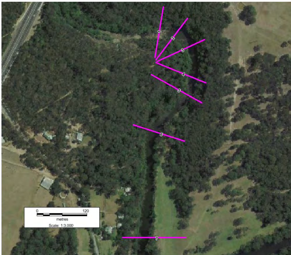
Figure 2: Upstream estimated cross section locations presented with aerial imagery
