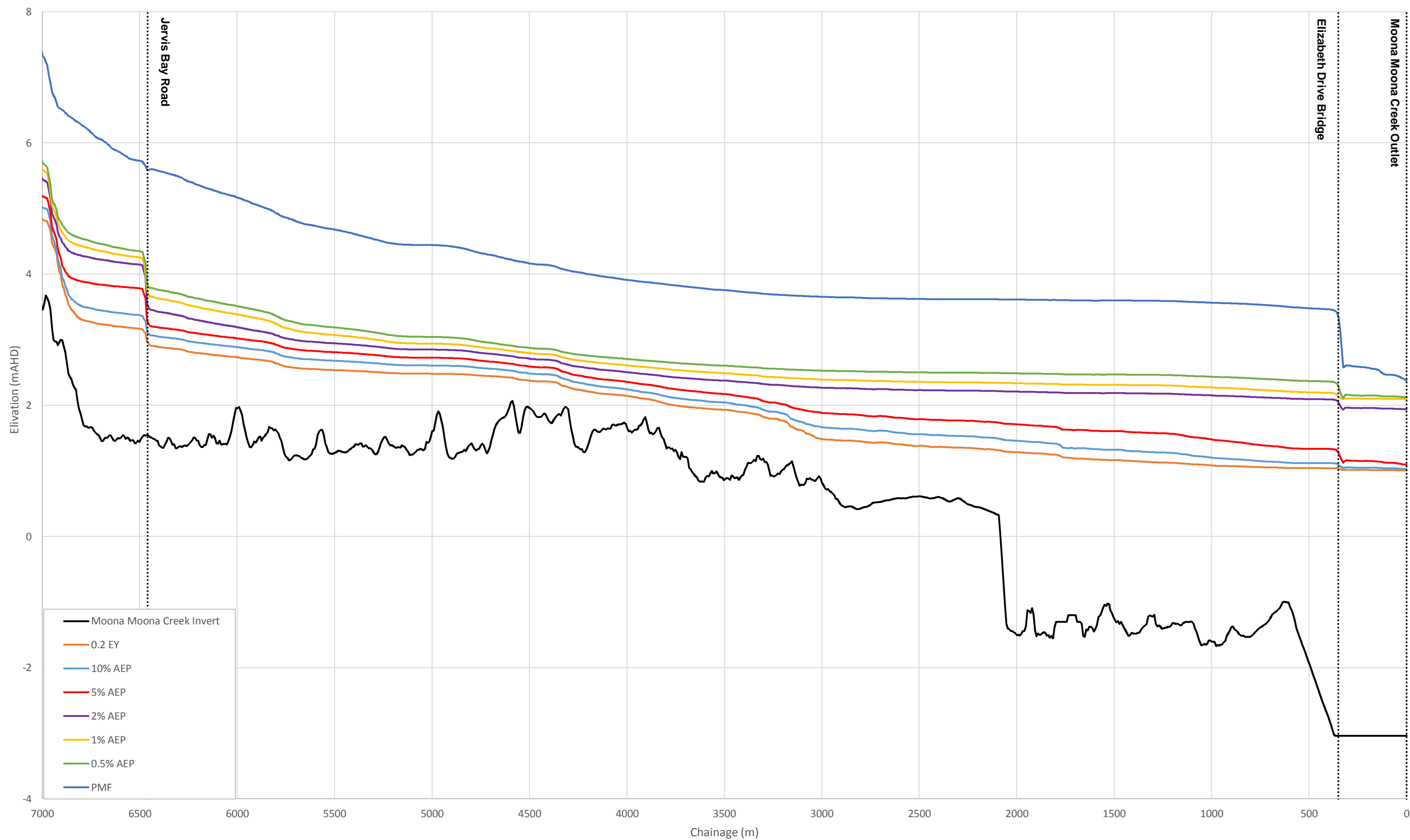
FIGURE 46 MOONA MOONA CREEK DESIGN FLOOD PROFILES
