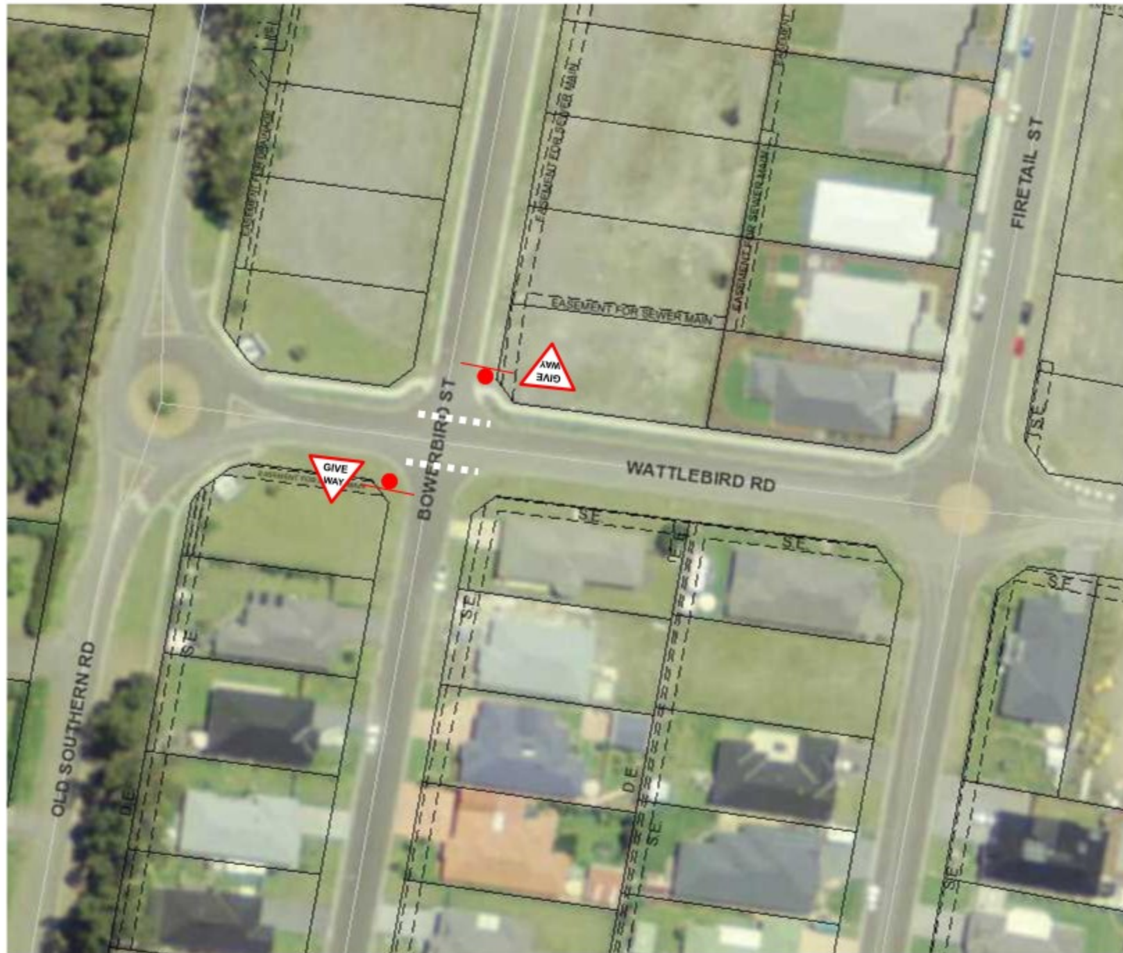
Proposed Give Way signs and hold lines intersection of Bowerbird St and Wattlebird Rd, Twin Waters Estate
