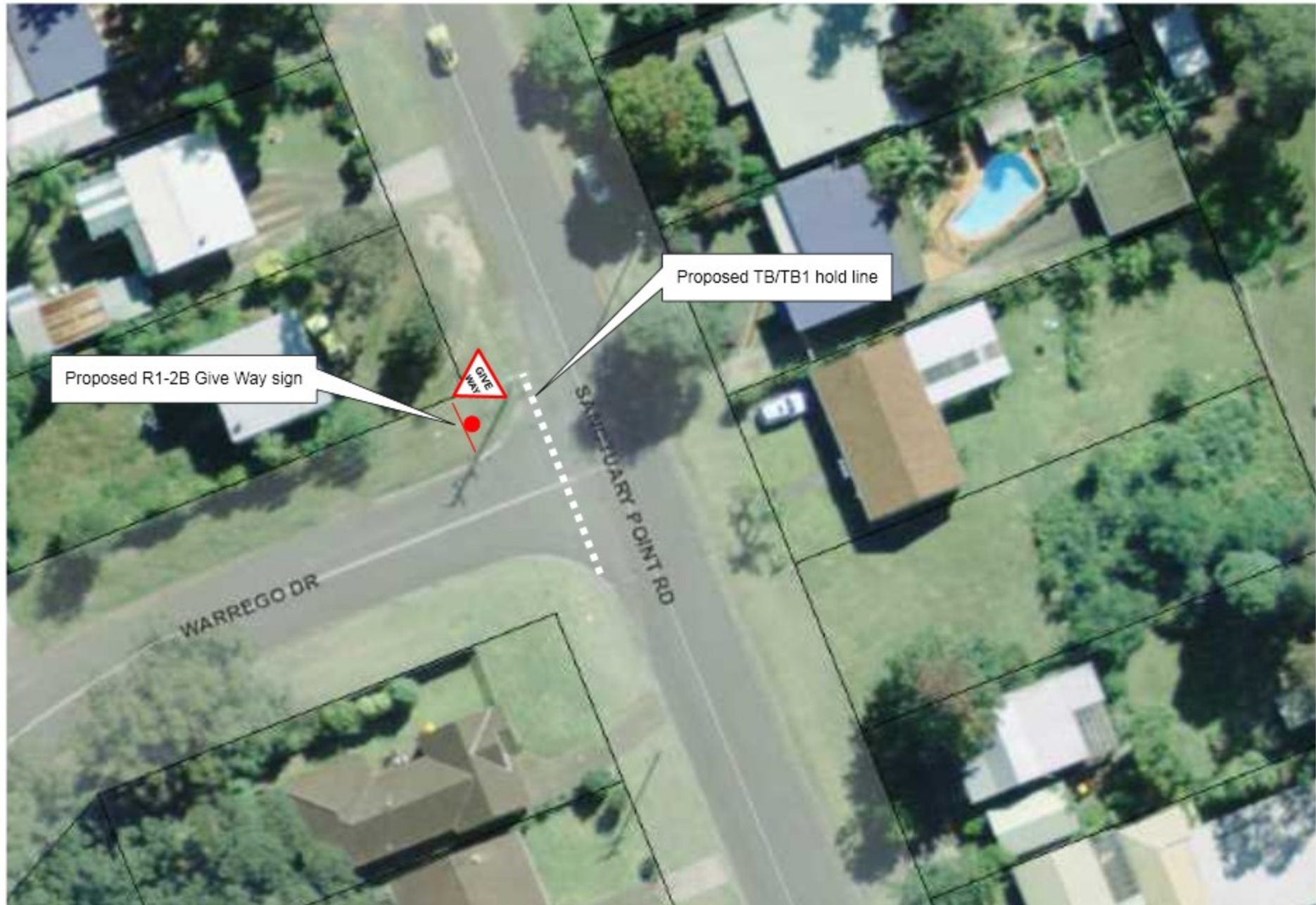
Proposed Give Way sign and associated hold linemarking intersection of Warrego Dr & Sanctuary Point Rd, Sanctuary Point
