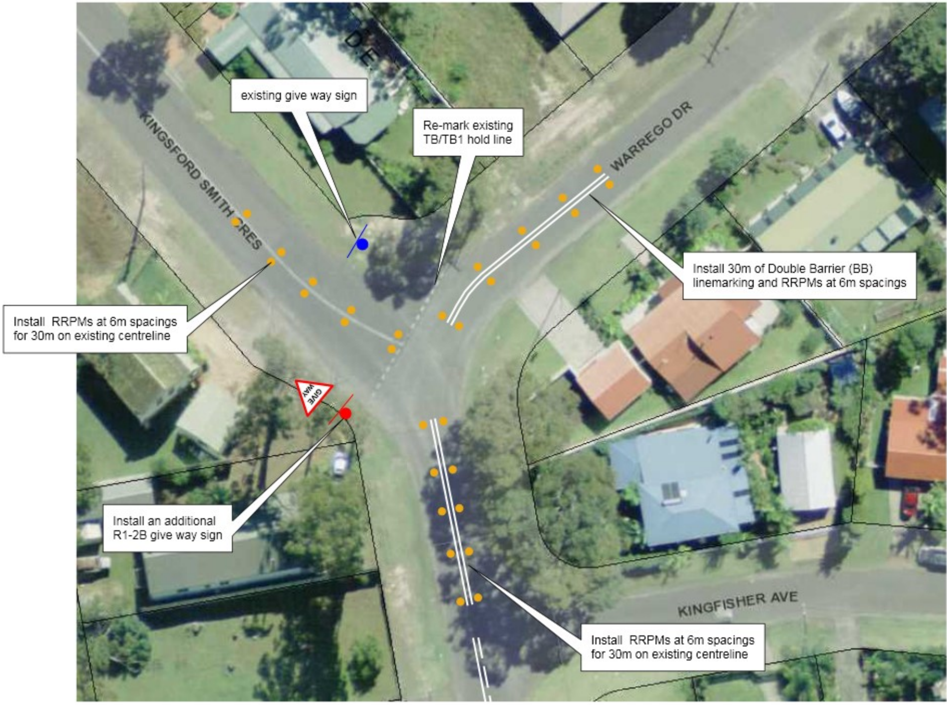
proposed signage and linemarking upgrade intersection of Warrego Dr/Kingsford Smith Cres, Sanctuary Point
