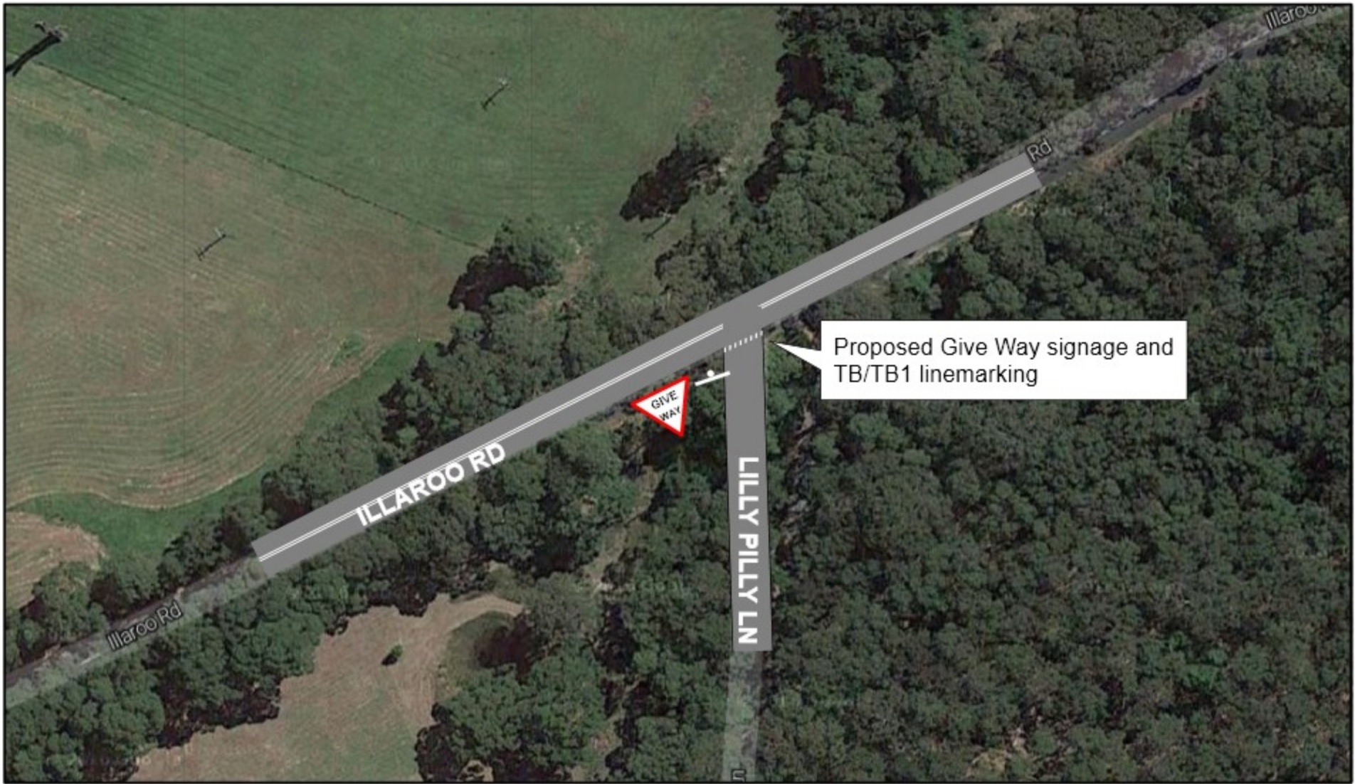
Proposed Give Way signage and associated linemarking Intersection of Illaroo Road and Lilly Pilly Lane, Tapitallee
