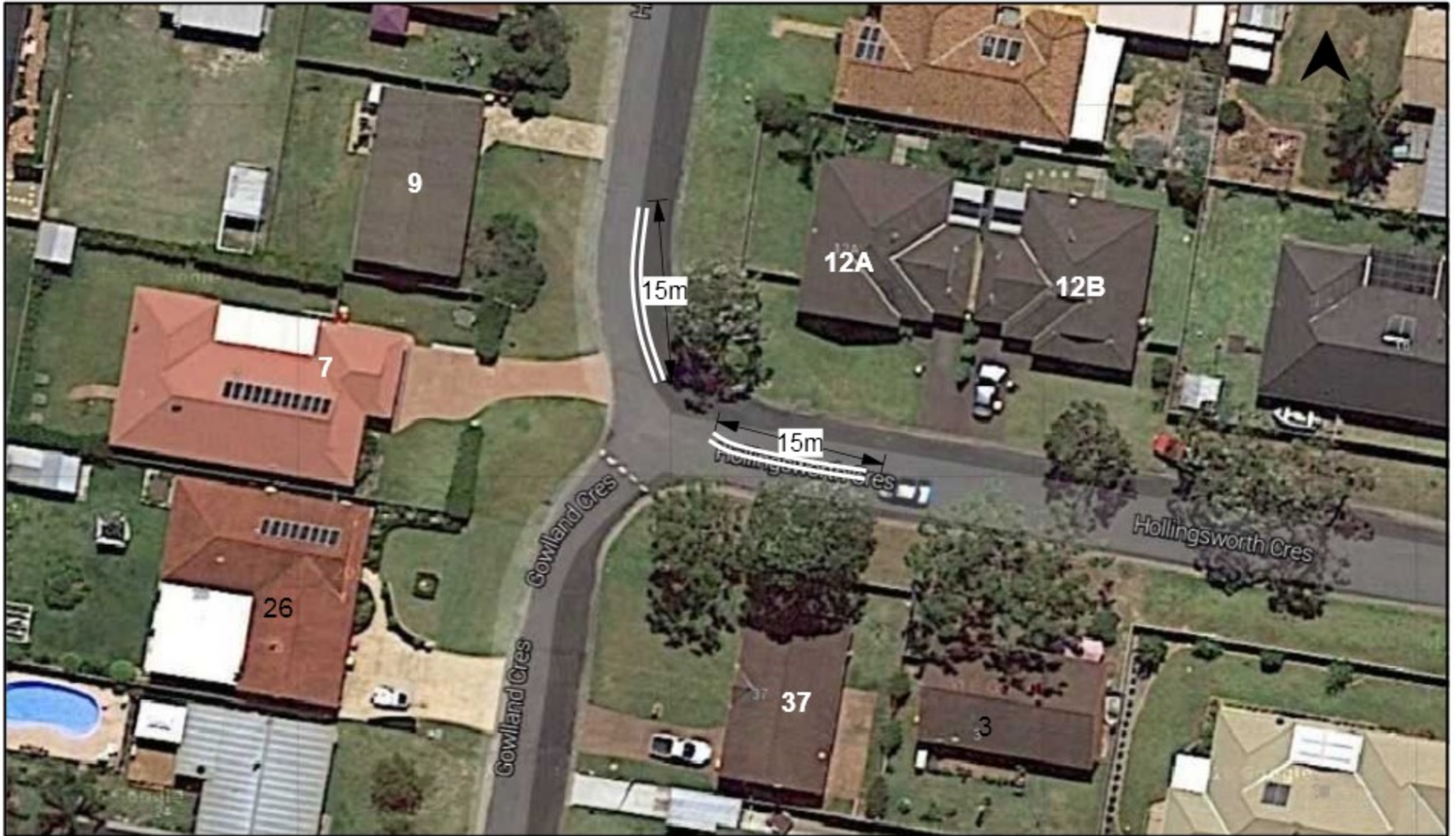
Proposed Double Barrier Line Marking Intersection of Gowlland Crescent and Hollingsworth Crescent, Callala Bay
