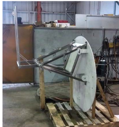
Two way tidal gate under construction at Council's Bomaderry Depot
