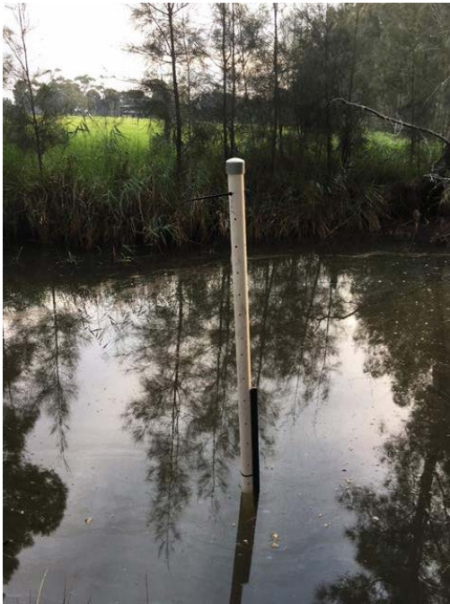
One of the four water level sondes installed in the drain
