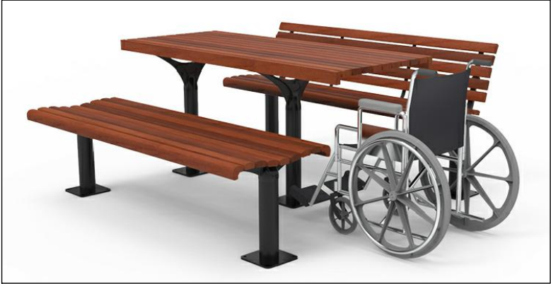
Botton & Gardiner - 'Urban Post Table' (AS1428.2) end access, Alugrain "Spotted Gum" slats and galvanised steel powdercoated 'Colorbond' "Monument" frame.
