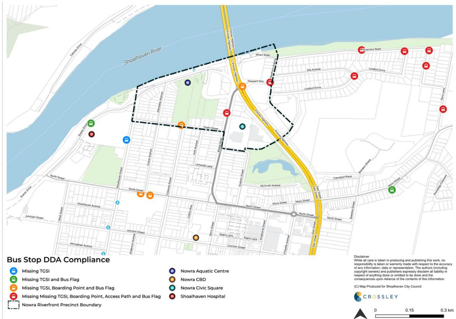
Figure 47: Location of DDA compliant bus stops (Source: Disability Standards for Accessible Public Transport 2002 and GTF5, 2021, modified by CrossleyTP 2022)
