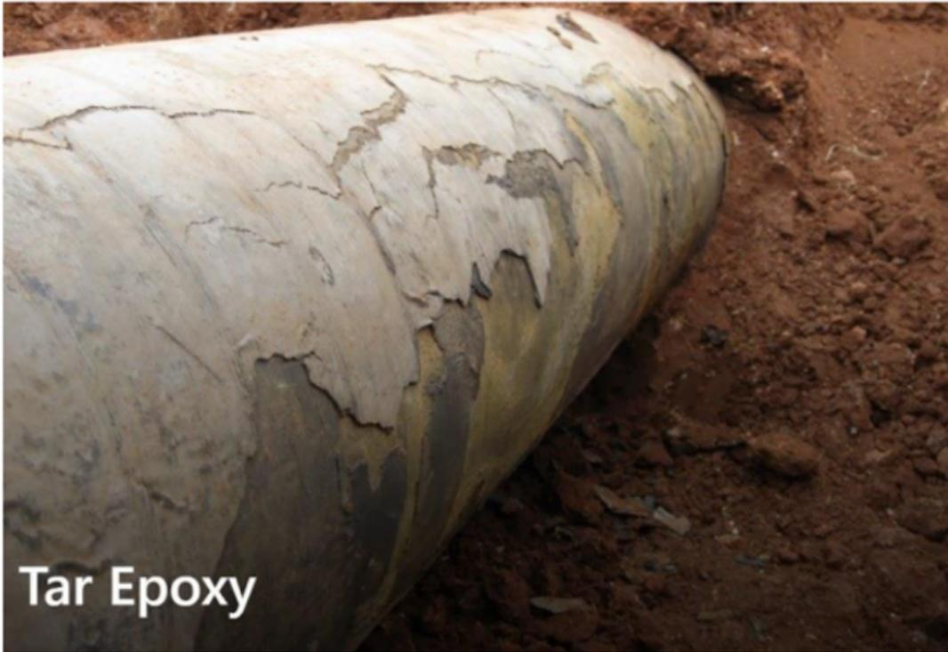
Figure 20 – Damaged asbestos coal tar coating at an unknown location. Note the remnant whitewash, spiral bandage wrap, black substrate.
