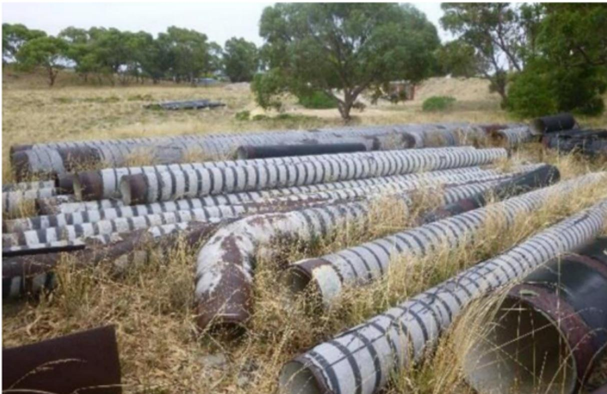
Figure 21 - Weathered asbestos coal tar coated pipe at Bold Park reservoir site. Note the spiral wrap and fading of the coating to a light grey.
