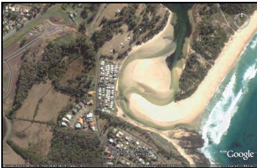
Figure 4 Early 2006 image showing westward growth of shoal and realignment / lengthening of ebb channel
