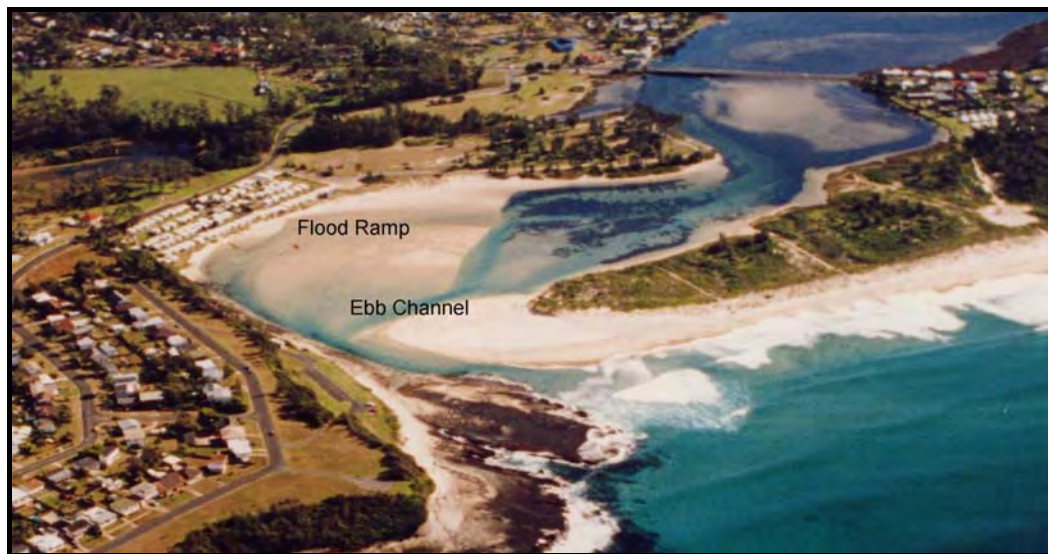
Figure 1 Typical entrance channel configuration (1993 photography)
