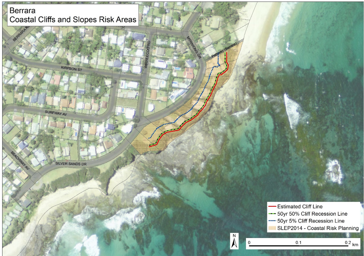
Figure 3.15 - Coastal Cliffs and Slopes Risk Areas Berrara
