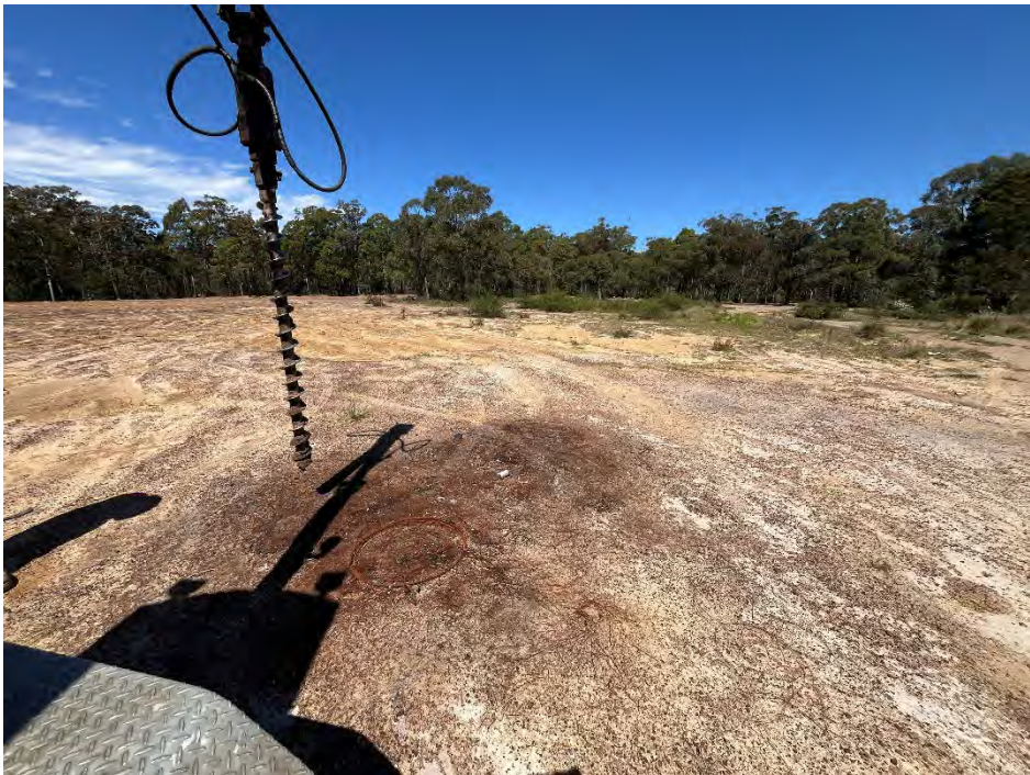
Photograph 19: Burnt stockpile where BH04 was drilled showing legacy scrap metal wire.
