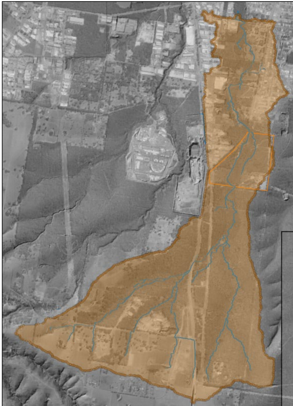
Figure 8: Catchment for rainfall data extraction
