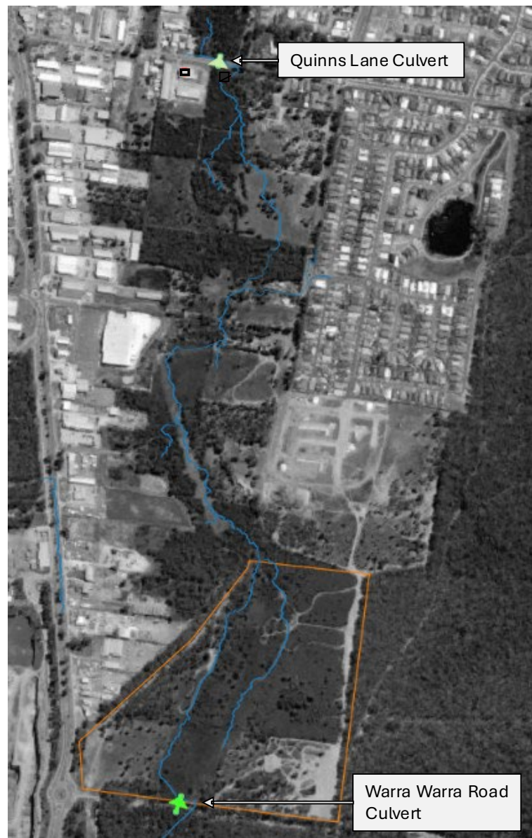
Figure 14: Culvert location (Pre-Development)
