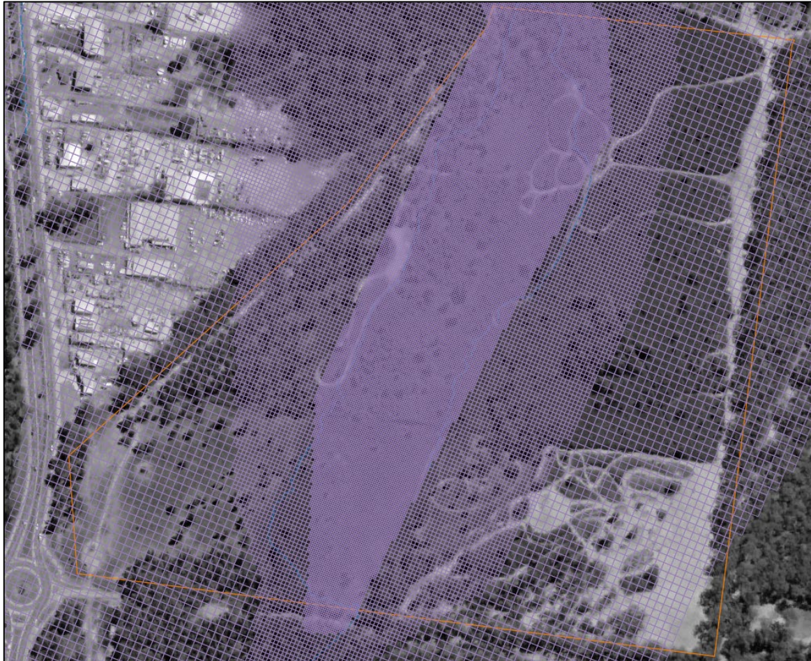
Figure 7: TUFLOW 2D model cell mesh
