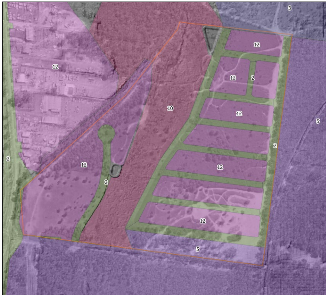
Figure 31: 2D Hydraulic Model – Manning's Roughness (Post-Development)
