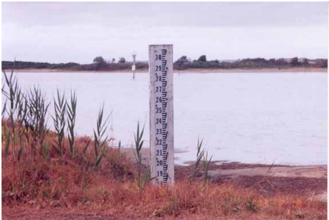
Figure 6. Water level indicators at River Road – gauge plate in foreground and automatic recorder in background.
