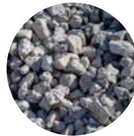
③ Recycled Concrete
