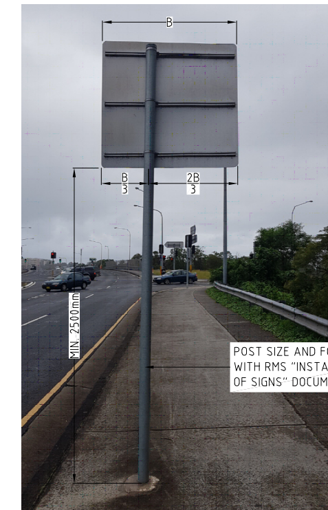
TYPICAL SINGLE POST SUPPORT TREATMENT FOR LARGER SIGNS
