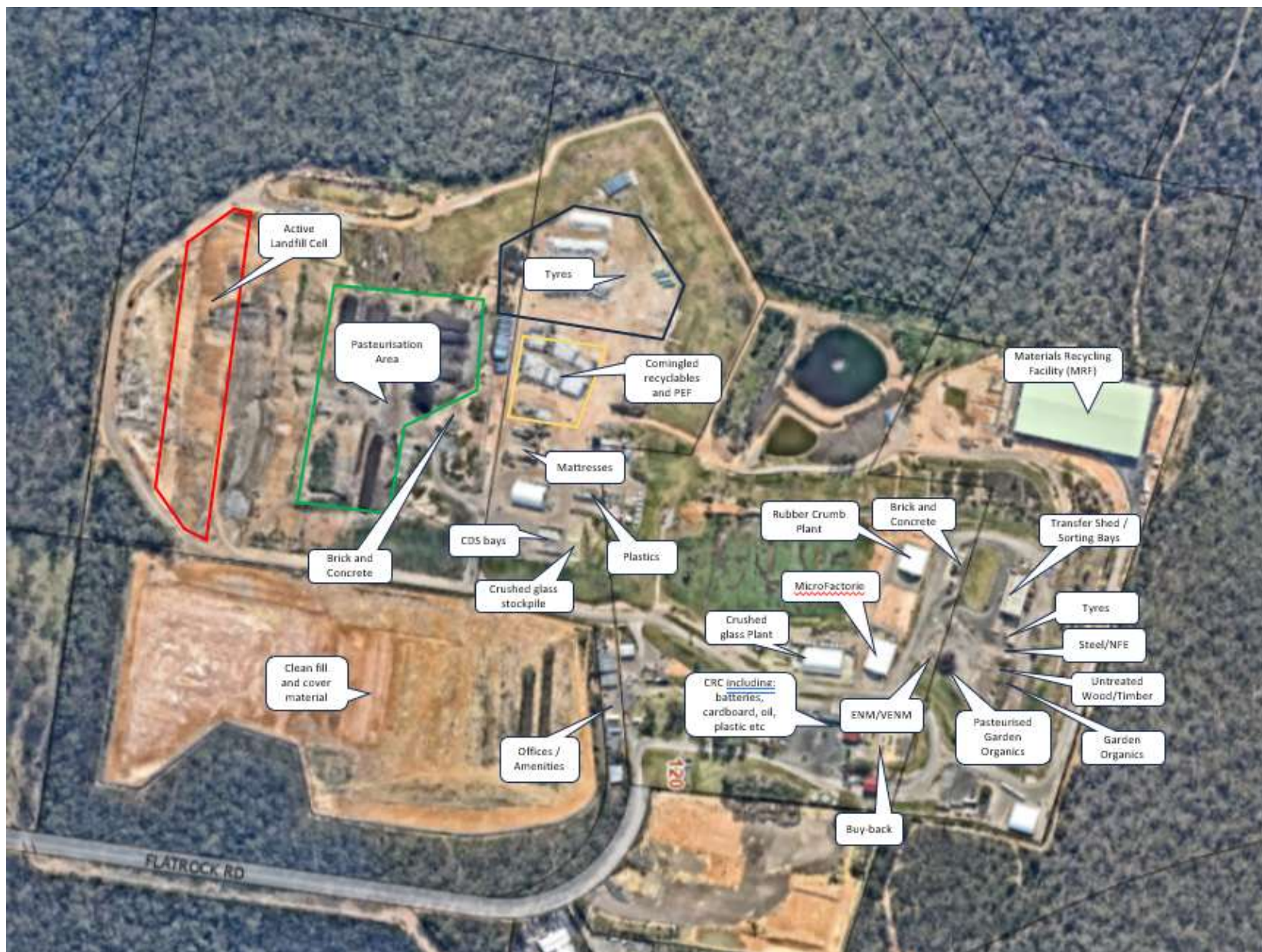
Figure 1: Site details and stockpile locations
