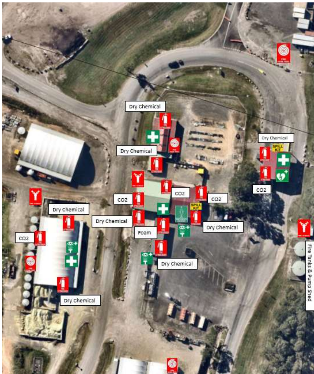
Figure 4: Site emergency equipment - buyback, weighbridge and glass plant
