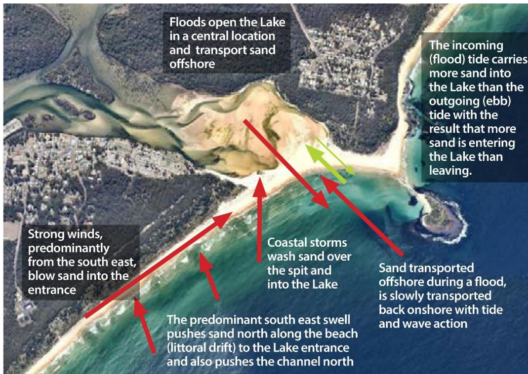
Figure 2-13: Simplified model of sedimentary processes at Lake Conjola entrance (from Coastal Fact Sheet, 2018)
