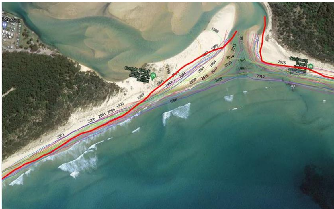
Figure 2-16: Selected plots of water line position along the beach near the entrance to Lake Conjola over the period 1990-2019 from satellite imagery
