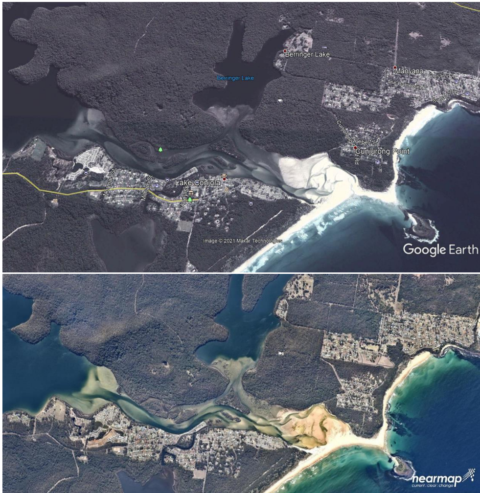
Figure 5-1: Loss of distinct ebb tide channel due to storm washover – September 2011 (top) and September 2018 (bottom)
