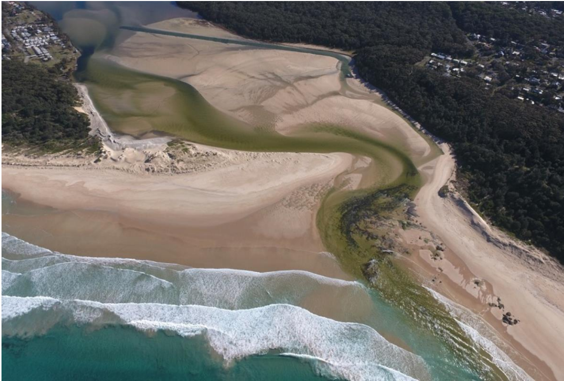
Figure 4-21: View looking westwards over the entrance area showing the dredged channel in the background and natural channel in the foreground (CCB, 2017)
