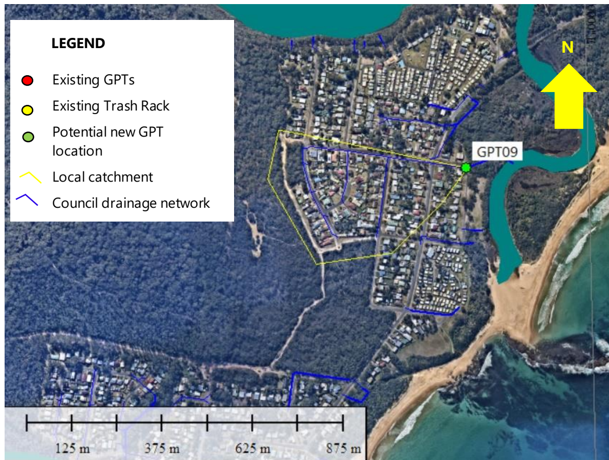
Figure 6-14 – Recommended GPT locations in Swan Lake area
