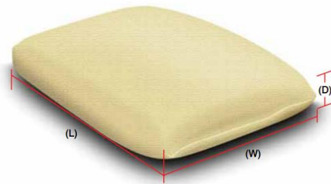
Figure 4-1 Schematic of an ELCOROCK GSC Unit
