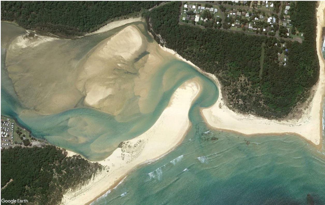
Figure 5-11: Aerial photograph showing an example of the Regime Entrance State (source: Google Earth Pro, dated 13 February 2016)
