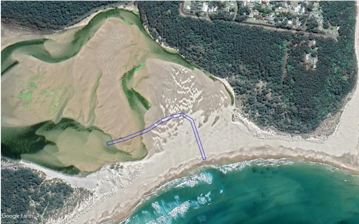
Figure 4-2: Indicative arrangement of longer pilot channel (400m length) in northern spit zone (source: Google Earth Pro dated 29 September 2018)
