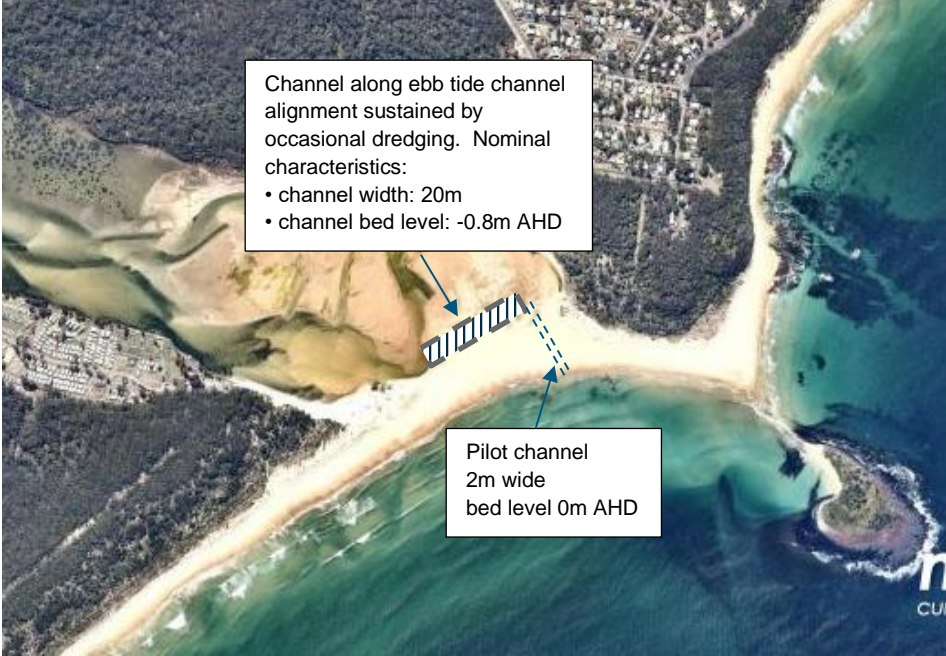
Figure 4-5: Indicative arrangement of ebb tide channel dredging
