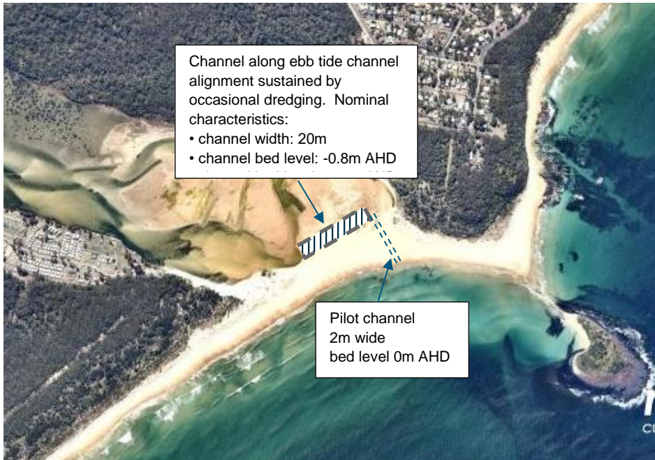
Figure 5-19: Diagram summarising the concept for Option 3 – air photo date 14 September 2018
