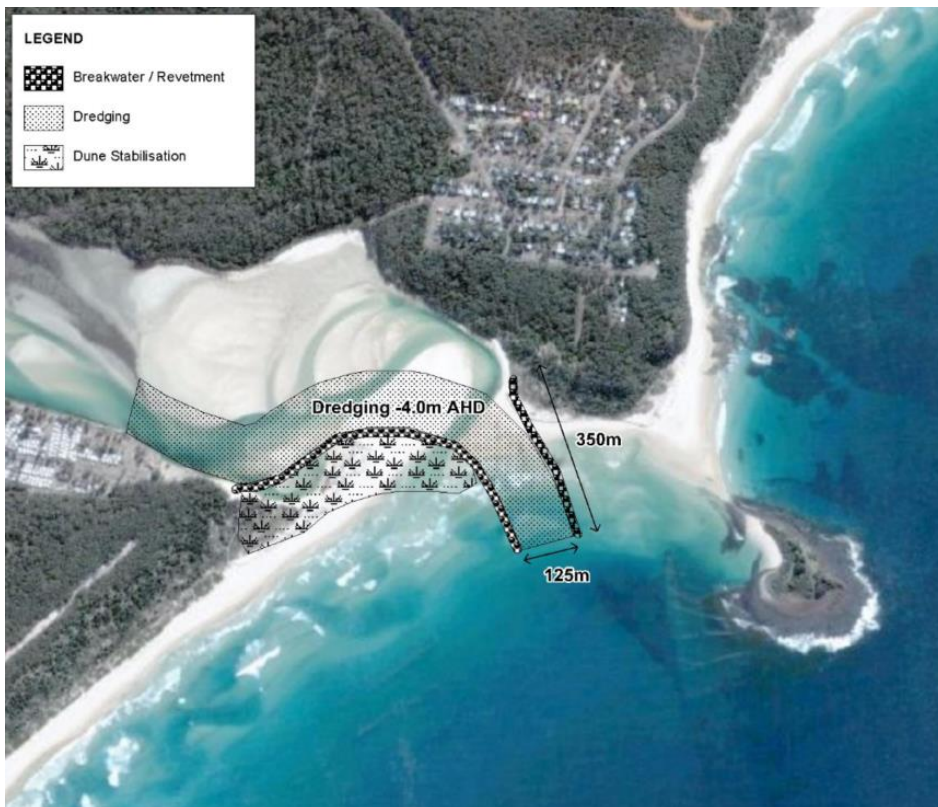
Figure 5-23: Conceptual arrangement for a permanent entrance adopted in BMT WBM (2013a)
