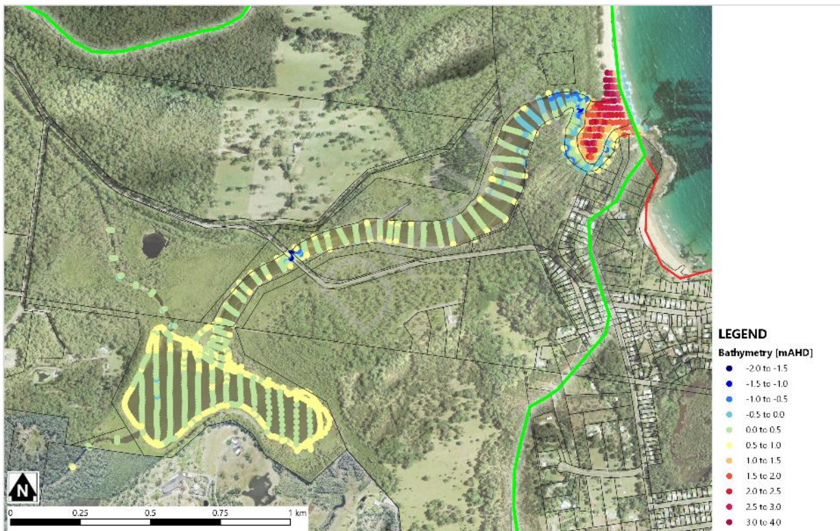
Figure 4-2 Bathymetric Survey Data (OEH, 2002)
