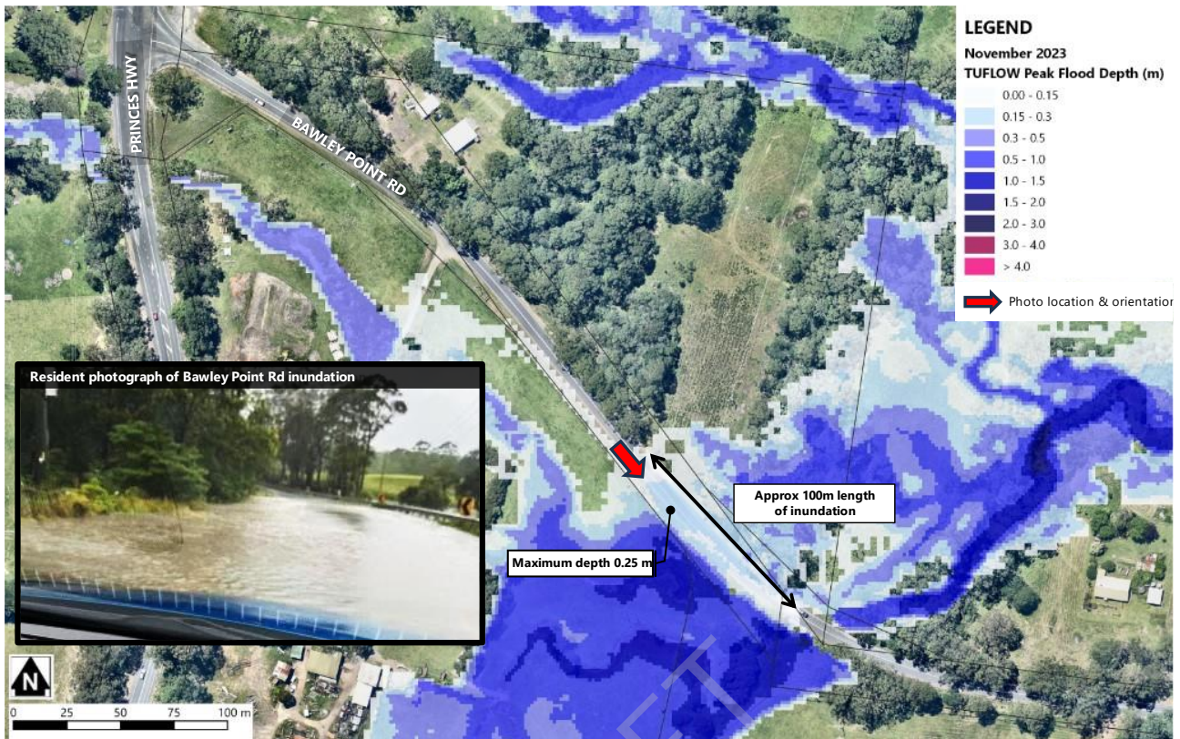
Figure 7-7 November 2023 event comparison of TUFLOW results to photograph
