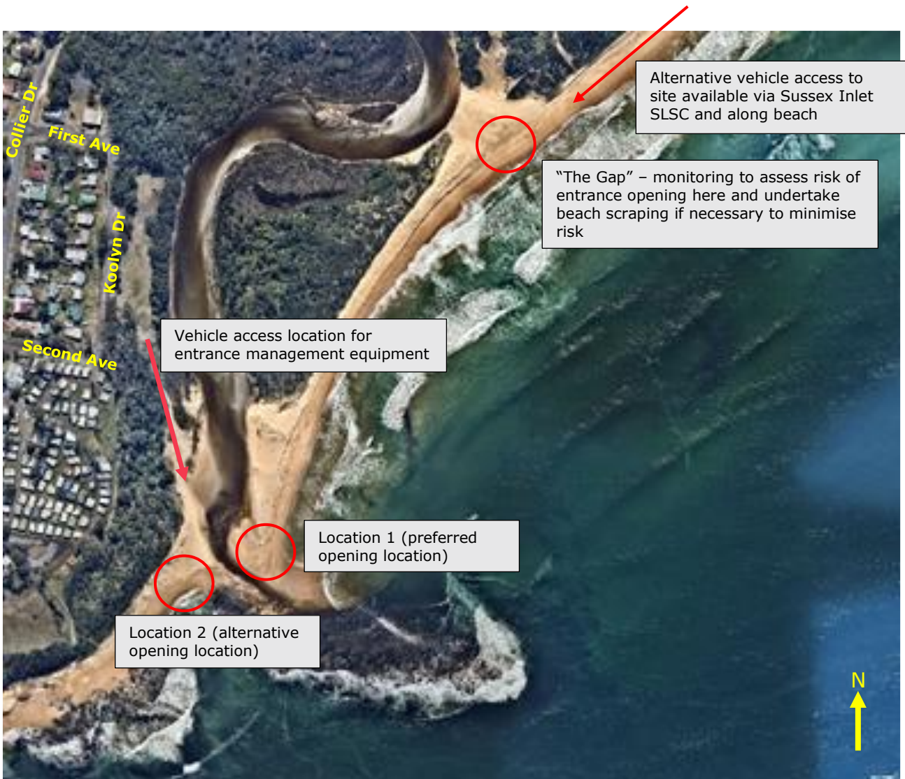
Figure 8-3 Locations where lake openings are possible. Locations 1 and 2 are specified as acceptable for planned openings by the Entrance Management Policy.
