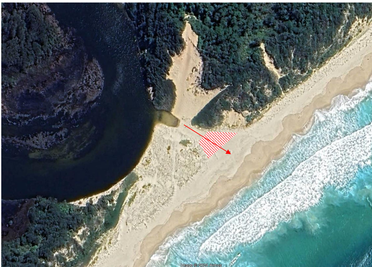
Figure 8-4 Recommended survey transect location through "The Gap" to assess berm levels and the potential for a breach. Beach scraping recommended to achieve berm level of 3.0m AHD or above within hatched area.
