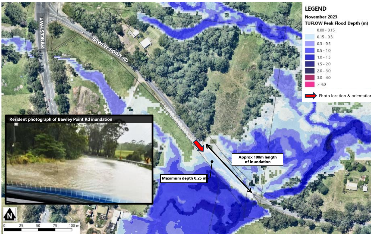
Figure 3-4 Comparison of model results to photo of Bawley Point Road near Princes Highway
