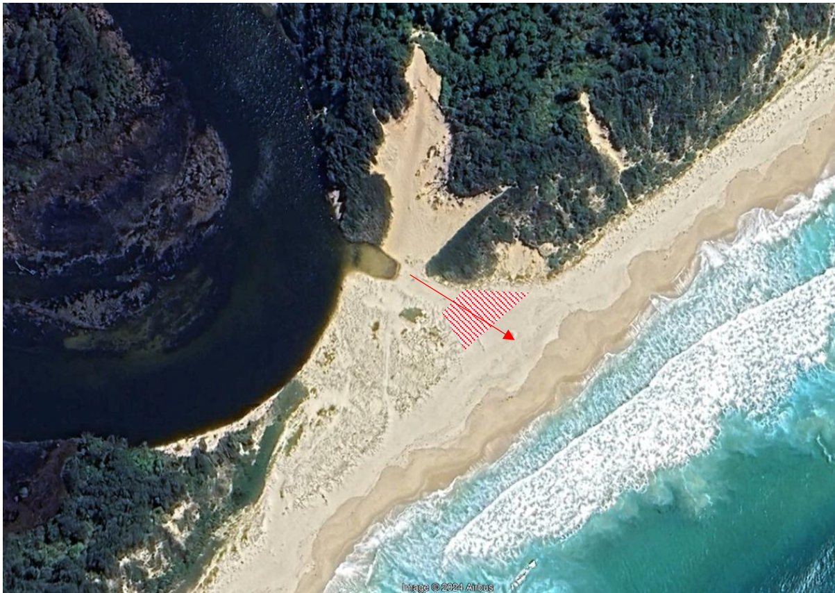
Figure 15 Recommended survey transect location through “The Gap” to assess berm levels and the potential for a breach. Beach scraping recommended to achieve berm level of 3.0m AHD or above within hatched area.
