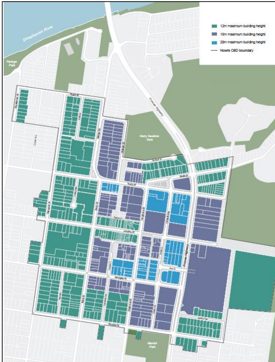
Figure 1 - Recommended Building Heights
