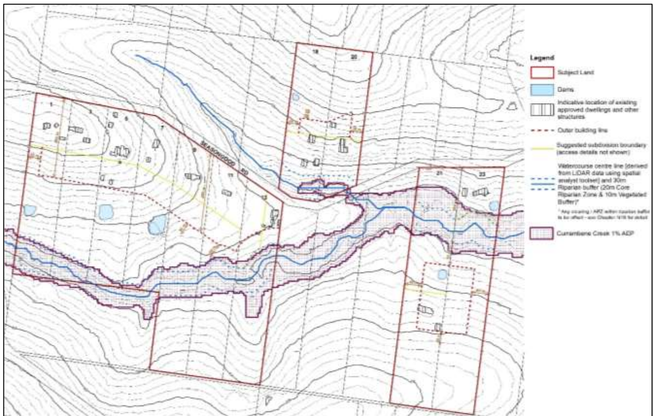
Figure 6 – Flood liable land (1% AEP) at Seasongood Road (Currumbene and Moona Moona Creek Flood Study, 2013)
