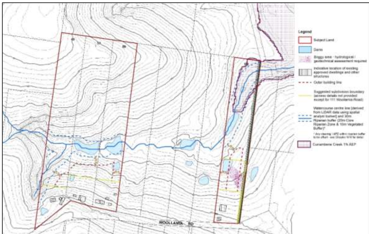
Figure 5 – Flood liable land (1% AEP) at Woollamia Road (Currumbene and Moona Moona Creek Flood Study, 2013)
