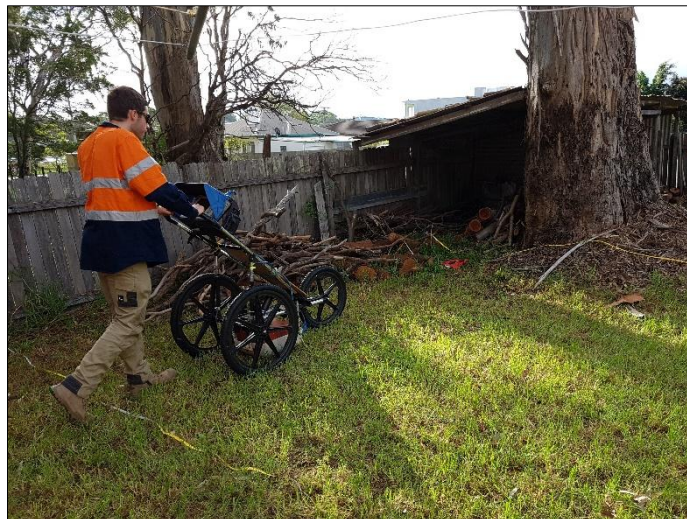
Figure 3. A section of the survey area with scan in progress. Tapes were used to ensure correct line separations and directions were achieved.
