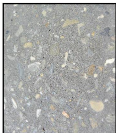
Honed Concrete Surface Finish
