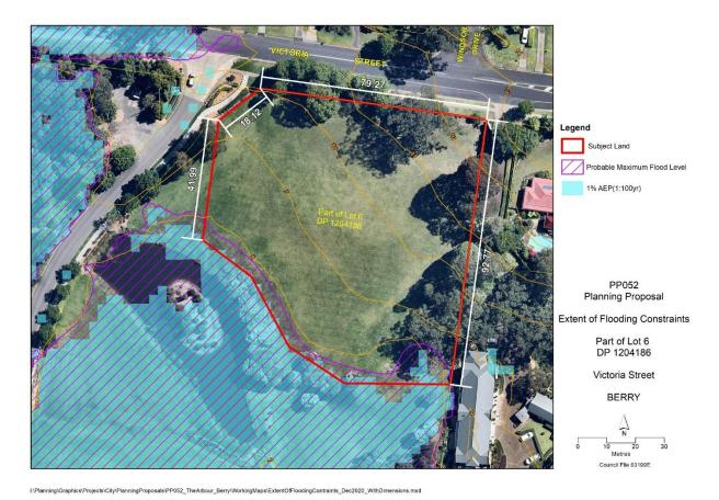
This diagram appears as Figure 1 – Extent of 1% AEP (1 in 100 year flood) and Flood Planning Level (FPL) (FPL = 1% AEP + 0.5 m freeboard) in the exhibited PP.
