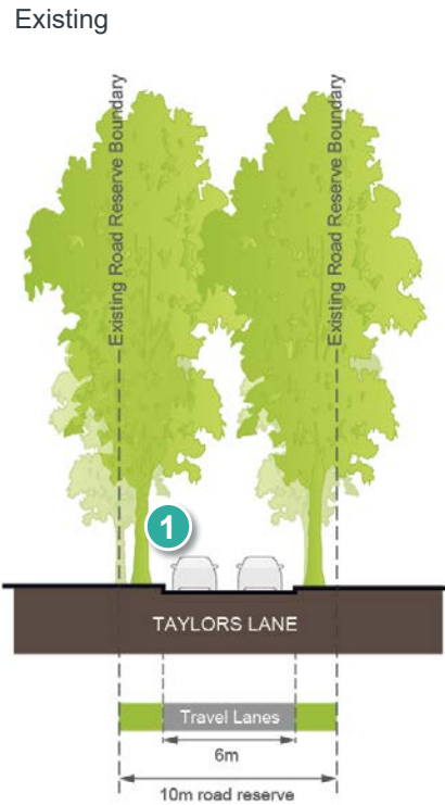
Figure 49 Street section - existing section
