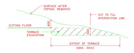
Figure C213.1 - Transition from Cut to Fill
