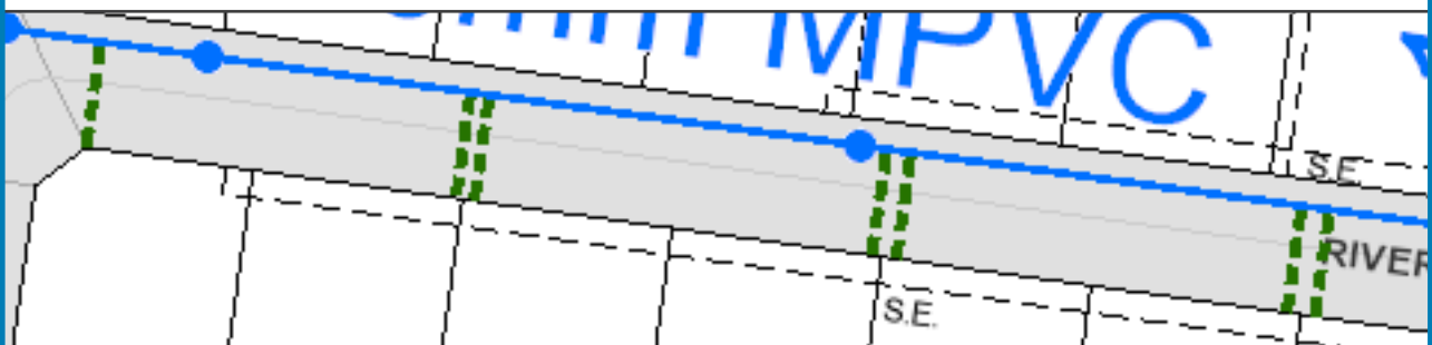
Example of conduit in place from the main water line. Note: the green line indicates existing conduit
