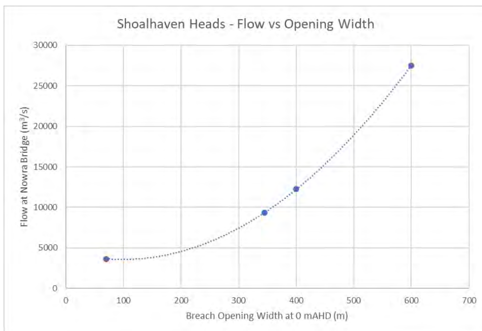
Figure 4-3 Relationship between flow at Nowra Bridge and Shoalhaven Heads breach opening width
