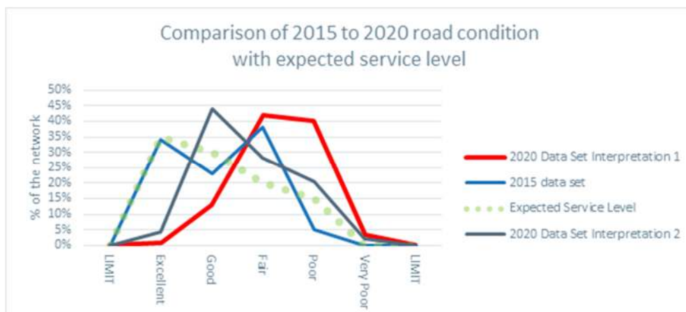
Figure 0.1 2020 Road Condition Report Extract
