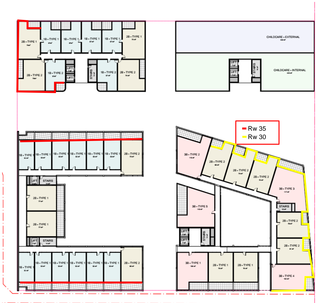
Figure 5-1 Typical Floor Rw Requirements
