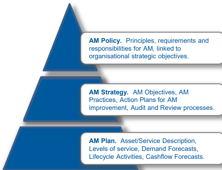
Figure 1: The Asset Management Framework (IIMM 2015)
