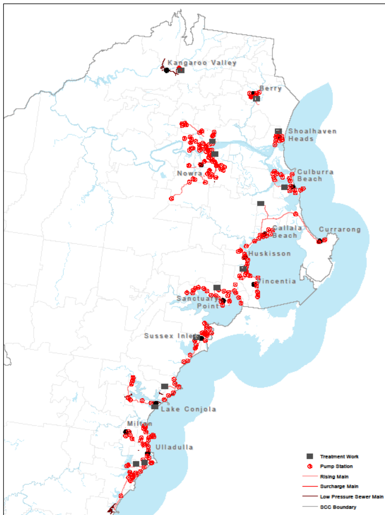
Figure 4-2 Shoalhaven Wastewater Network
